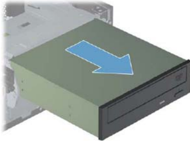
Figure 8-18 Removing the optical drive
