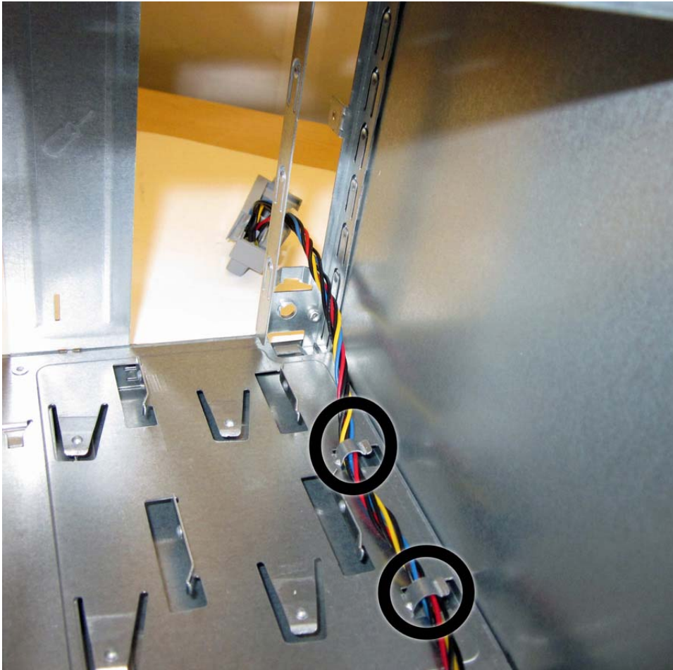
Figure 7-39 Power switch cable routing
