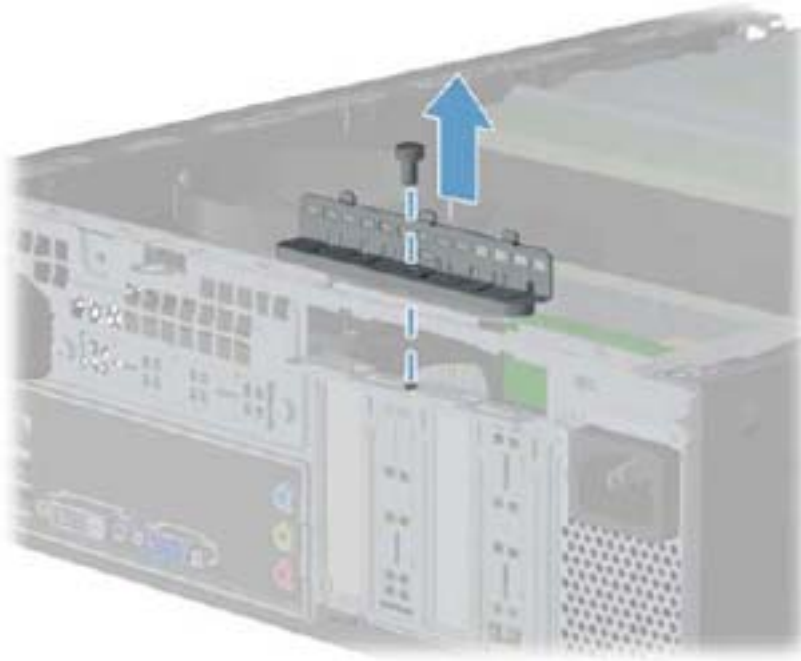
Figure 8-11 Opening the expansion slot bracket
