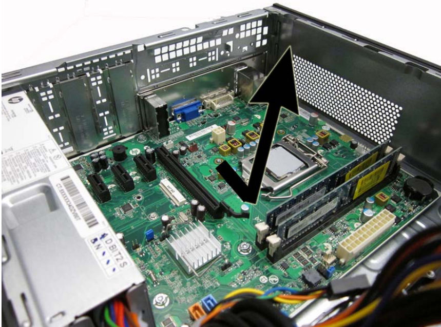
Figure 8-39 Removing the system board
