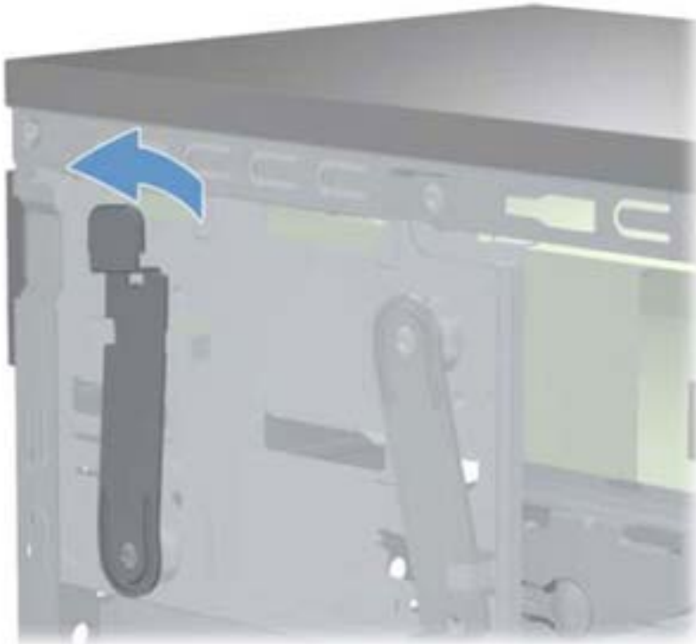
Figure 7-21 Pushing the optical drive
