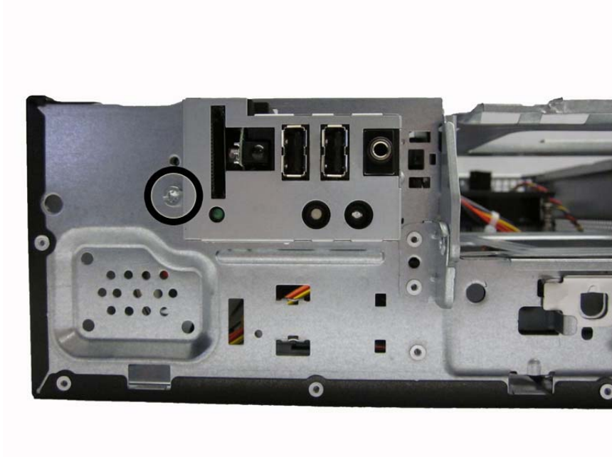
Figure 8-29 Removing the front USB assembly screw
