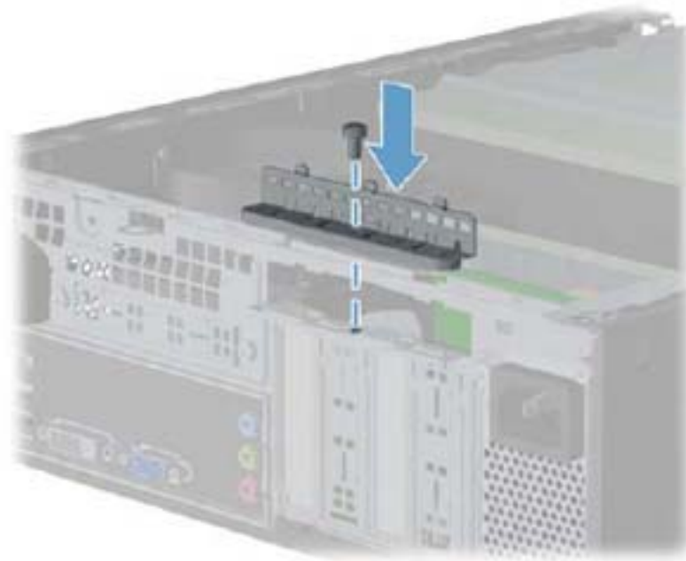
Figure 8-14 Replacing the expansion slot bracket
