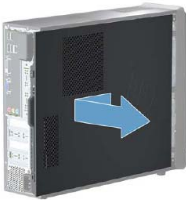
Figure 8-2 Removing the access panel
