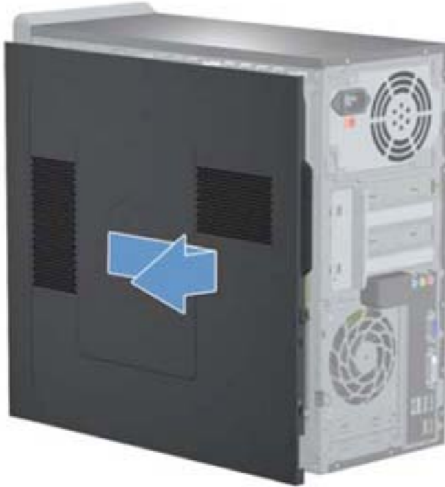
Figure 7-2 Removing the access panel
