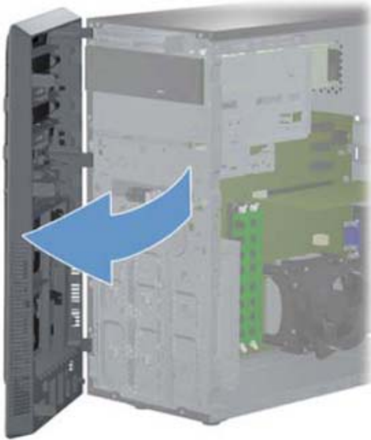
Figure 7-4 Removing the Front Bezel
