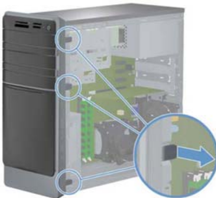
Figure 7-3 Removing the Front Bezel
