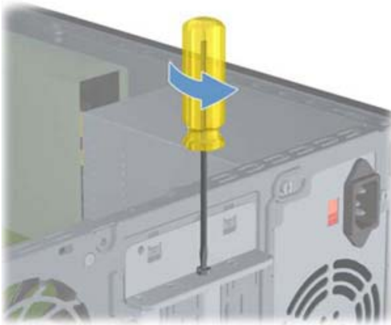
Figure 7-11 Opening the slot cover lock
