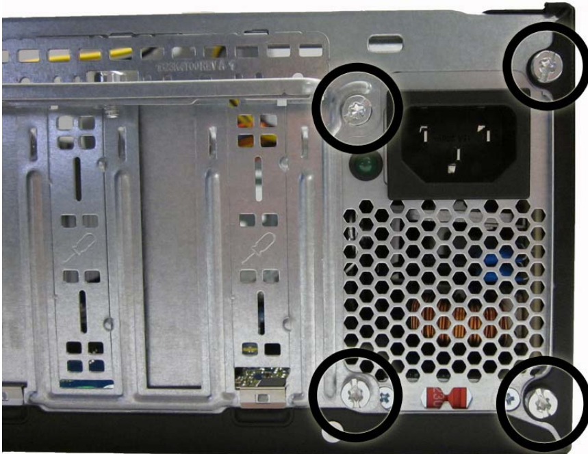
Figure 8-36 Removing the power supply screws
