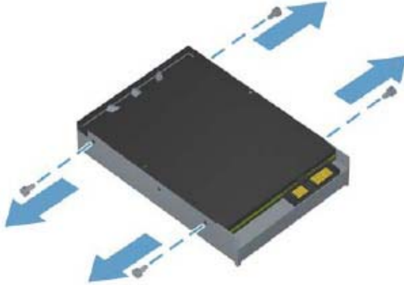
Figure 8-23 Removing the hard drive guide screws
