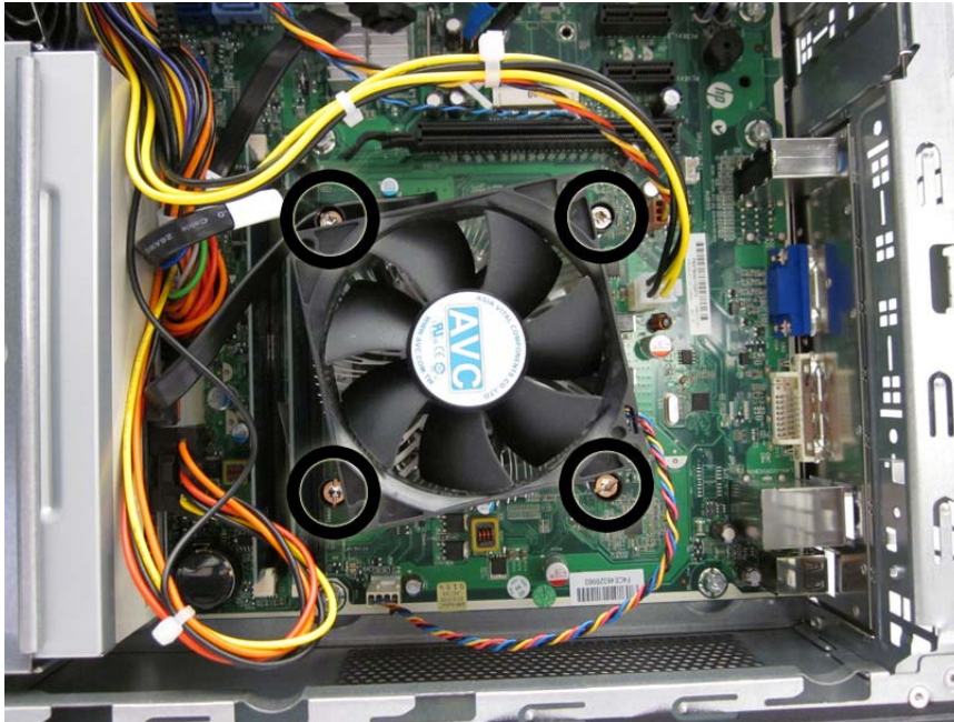
Figure 8-33 Loosening the fan sink screws
