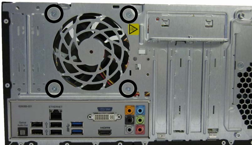
Figure 7-41 Removing the fan
