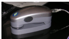
Calibration position for Eye-One Pro/Monitor
