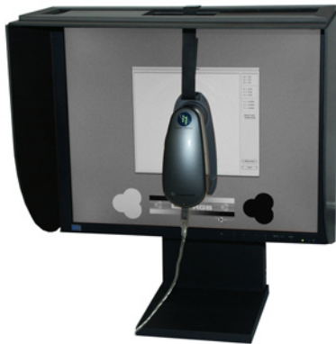
LCD-flat screen with ambient light hood and Eye-One Pro spectrophotometer.
