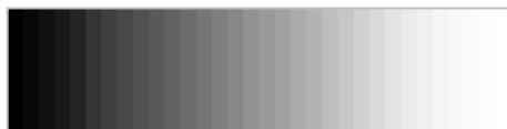
Software-calibrated monitor: Depending on the quality of the monitor, not all steps may be distinguishable, especially in highlights and/or shadows
