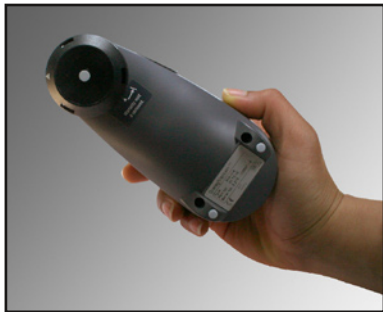
Positioning of the GretagMacbeth Eye-One Pro for ambient light measurement
