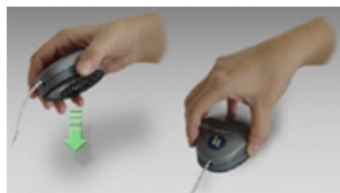
Calibration position for the basicColor SQUID/Eye-One display
