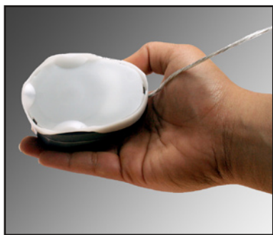
Positioning basICColor SQUID2 for ambient light measurement.
