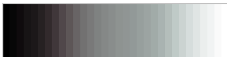
Uncalibrated monitor: The tonal distribution is irregular and the grays show a color cast.
