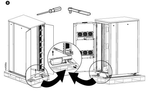
9. Remove the bolt securing the ramp bracket (A) attached to the pallet. Remove the bolt securing the second ramp bracket (**B**) which is installed on the ramp. Extra ramp bolts are provided on the pallet and ramp.
