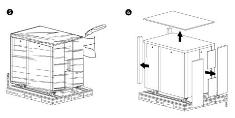
3. Once the plastic wrap has been removed, the foam corner protectors can be removed.
