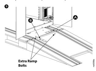
10. Close the doors. Secure the ramp to the pallet using the brackets and provided bolts.
