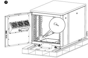
8. Unlock and open the front door. Remove the two (2) T-30 Torx screws securing each bracket to the rack. Use a 13 mm socket (not provided) to remove the two (2) 10 x 20 bolts securing each bracket (front and rear) to the pallet.
