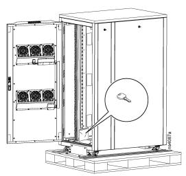
8. Unlock and open the front doors. Remove the two (2) T-30 Torx screws securing each bracket (front and rear) to the rack. Use a 13 mm socket to remove the two (2) 10 x 20 bolts securing each bracket to the pallet.
