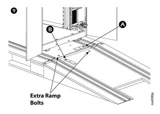
10. Close the doors. Secure the ramp brackets to the ramp and pallet using the provided bolts.
