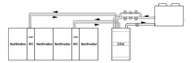
The CDU also provides the flexibility to pipe the main supply and return connections from the chiller from the top (overhead) or the bottom (from a raised floor), regardless of the distribution piping configuration. The CDU will ship with two brass counter flanges for connection of copper mains and two dielectric flanges for connection to steel piping.
