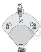
All the slave units will fire at the same output and be controlled to obtain a standard exposure.
