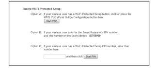
Push button: You may push the WPS button on the web menu or use the physical button on the back of the Smart Repeater.
