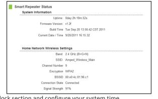
Home Wireless Network Settings: This section displays the current status of the connection between the High Power Smart Repeater and your Home Network. When viewing this section it is important to check that your Home Network SSID is correct, that the channel number matches your Home Network's channel number settings.
