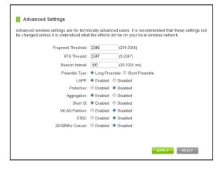
RTS Threshold: Adjusts the size of RTS data packets. Lower values reduce throughput, but allow the system to recover quicker from interference/collisions. Higher values provide the fastest throughput.
