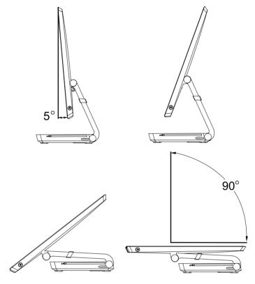
Use the stand to position the display to your preference. It can be rotated  $5^{\circ}$ forward and 90° backward.
