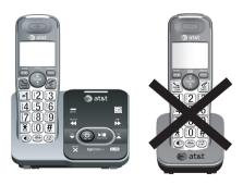
For registration, put the handset on the telephone base, not the handset charger.
