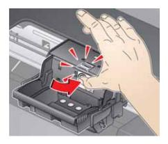
10. Insert the black ink cartridge into the printhead.
