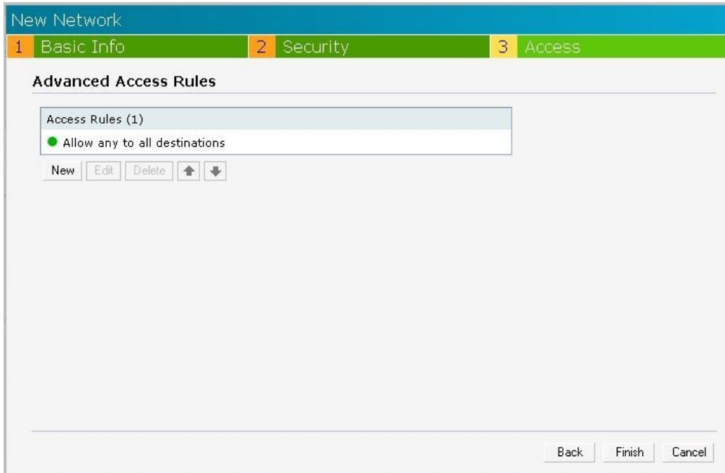
Figure 30 Adding an Employee Network – Access Rules Tab
