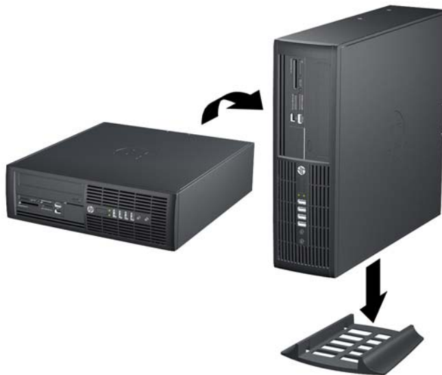
Figure 6-55 Changing from Desktop to Tower Orientation
