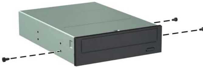
Figure 6-22 Installing Mounting Screws in the Optical Drive
