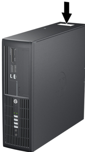
Figure 6-1 Serial Number and Product ID Location
