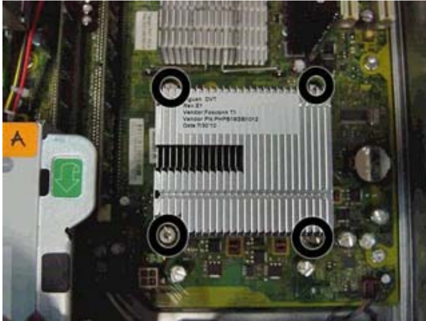
Figure 6-48 Removing the heat sink
