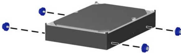
Figure 6-39 Installing Hard Drive Mounting Screws
