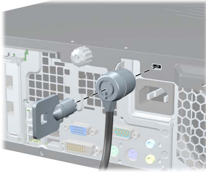
Figure 6-56 Installing a Cable Lock
