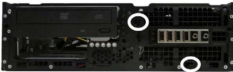
Figure 6-42 Front fan tab locations
