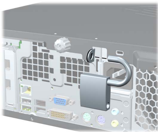
Figure 6-57 Installing a Padlock
