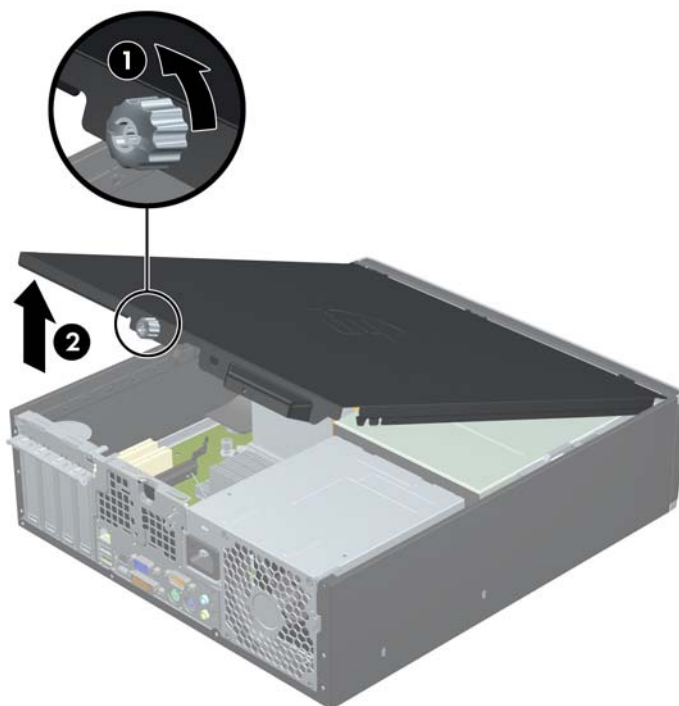
Figure 6-2 Removing the Access Panel
