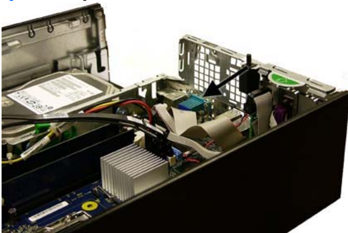
Figure 6-44 Removing the hood sensor from the chassis fan
