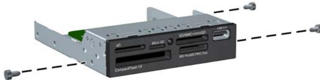
Figure 6-31 Installing Mounting Screws in the Media Card Reader
