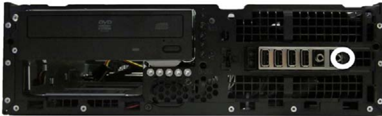
Figure 6-45 Removing the front I/O, power switch/LED assembly screw
