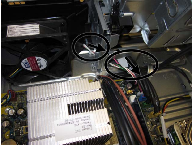
Figure 6-46 Routing the cables and removing the power switch assembly
