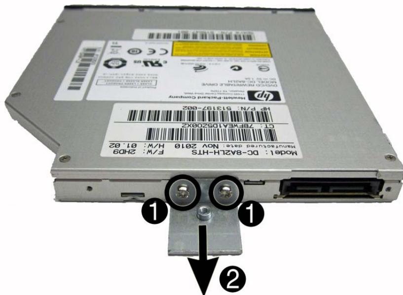
Figure 6-12 Removing the optical drive bracket
