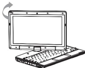
3. Follow the sign to turn the screen clockwise up to 180 degree so that the screen is facing out.
