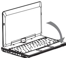
5. When done with Tablet PC, reverse the screen to 90 degree, turn counter set T1000/T1005 back to original posi
