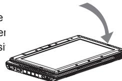
\* Attention: Please note that the screen can only rotate at 180 degree clockwise. Be sure to turn the screen according to the sign. Forcing the screen to turn at the wrong angle will cause serious damage to the the T1000/T1005.
