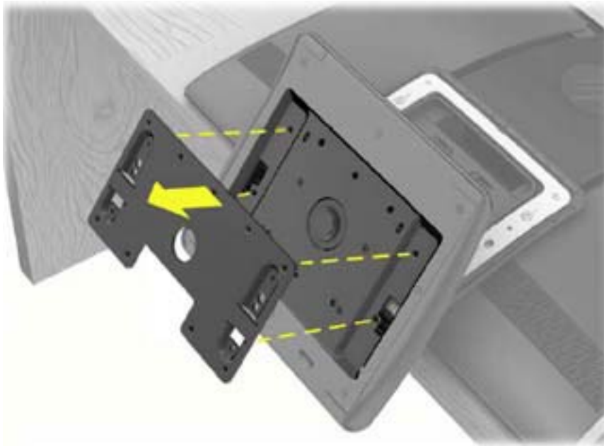
Figure 7-6 Removing the VESA adapter plate
