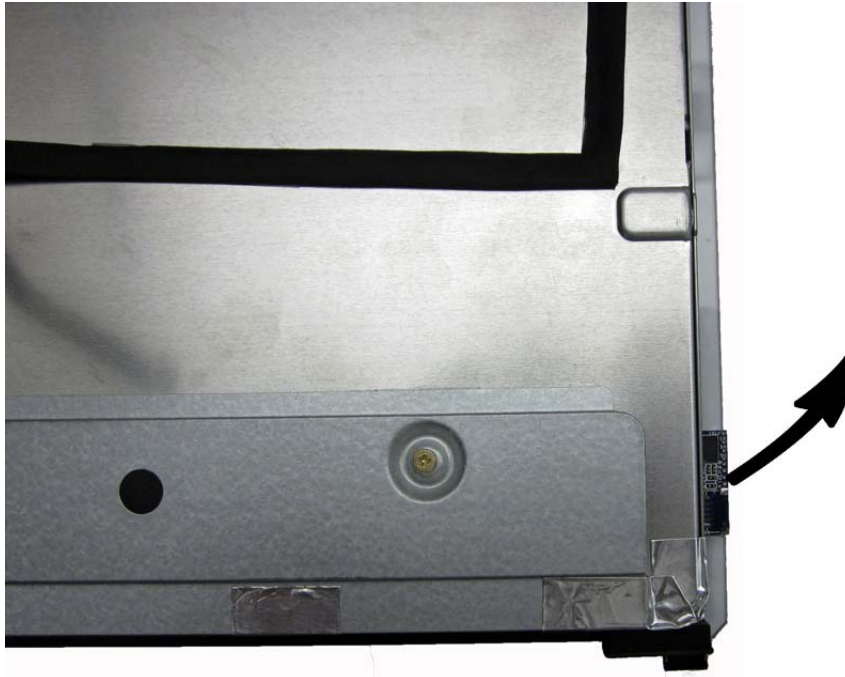
Figure 7-76 Removing the G-sensor board
