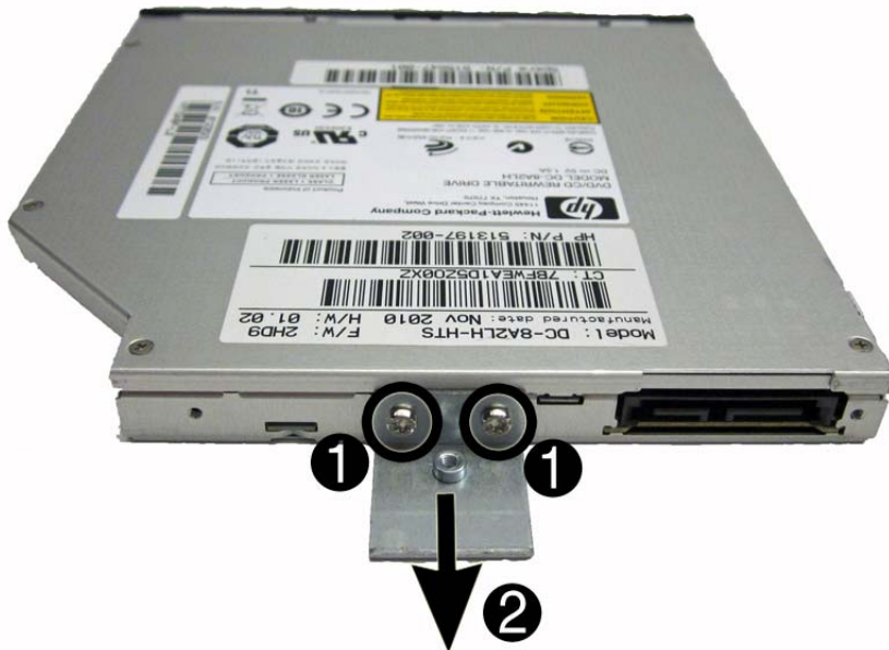
Figure 7-36 Removing the optical drive bracket
