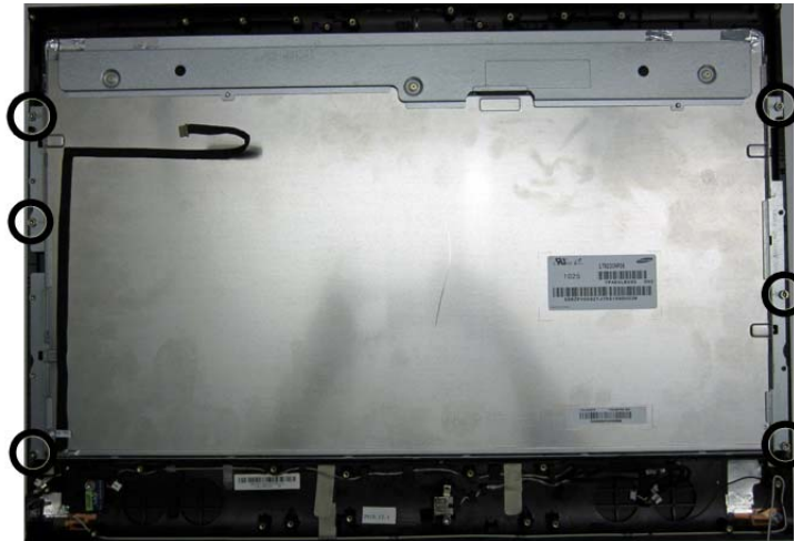
Figure 7-74 Separating the display panel from the front bezel
