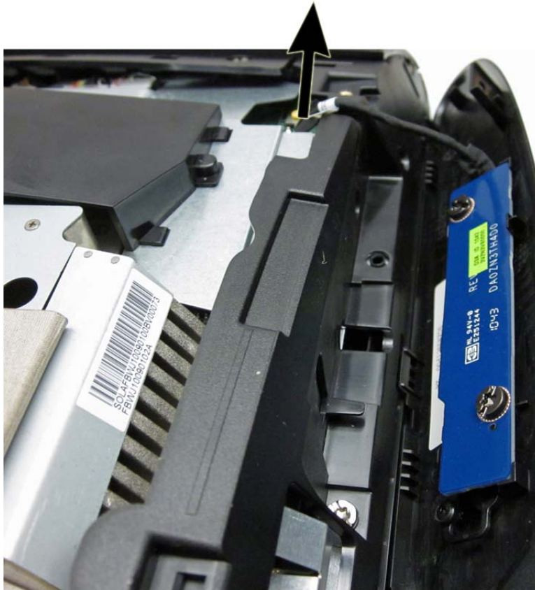
Figure 7-42 Disconnecting the volume board cable
