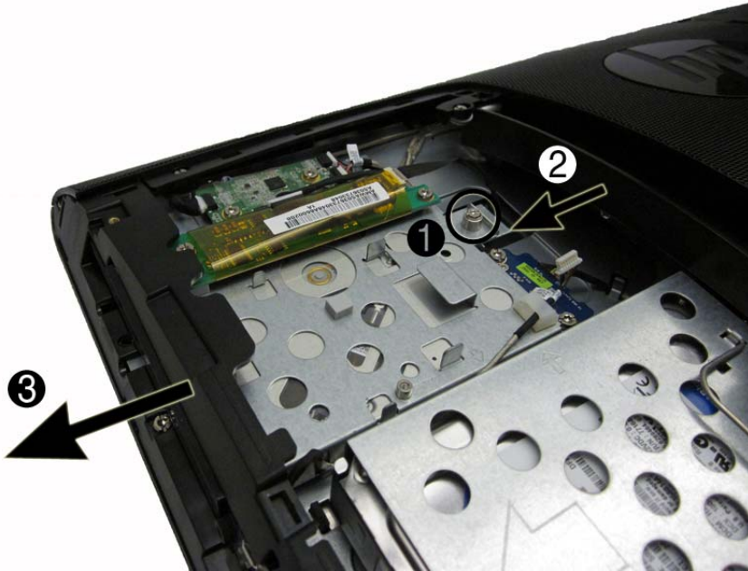
Figure 7-35 Removing the optical drive
