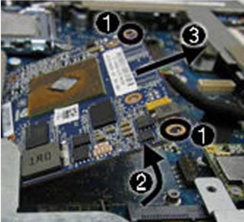
Figure 7-67 Removing the graphics board (board appearance may vary)
