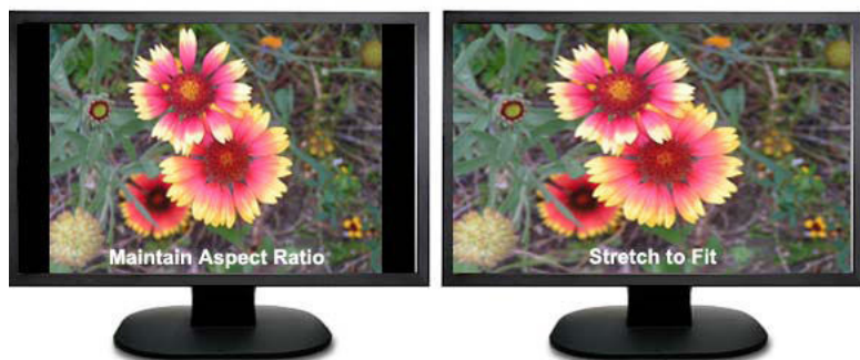
FIG. 104 Example of displays set to Maintain Aspect Ratio and Stretch to Fit
