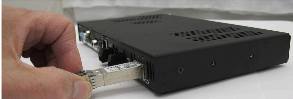
FIG. 63 Insert transceiver into transceiver socket
