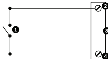
Figure 6.1 N.O. - Normally Open Non-supervised Connections
