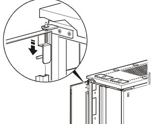
2. Using an Allen wrench, remove the door bumpers at the top and bottom of the door frame.
