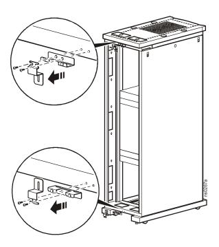
3. Using a Phillips head screwdriver, remove the rear door hinges and the rear skirt from the enclosure.
