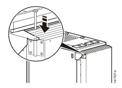
4. Align the upper hinge of the mounting frame with the upper hinge of the fan assembly, and slide the hinge pin into position.
