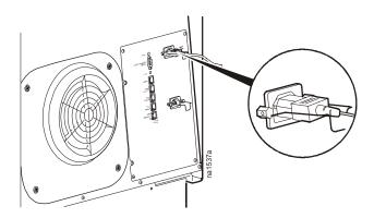
3. To provide redundant power to the unit, use the  ${\bf B}$  input socket to connect the ARU to a second source of protected power.
