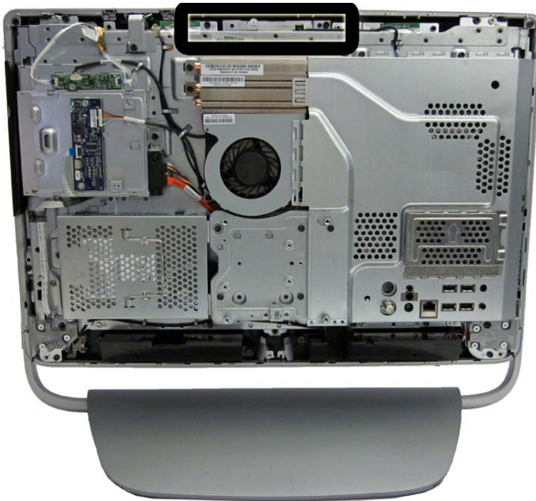
Figure 7-17 Webcam module location
