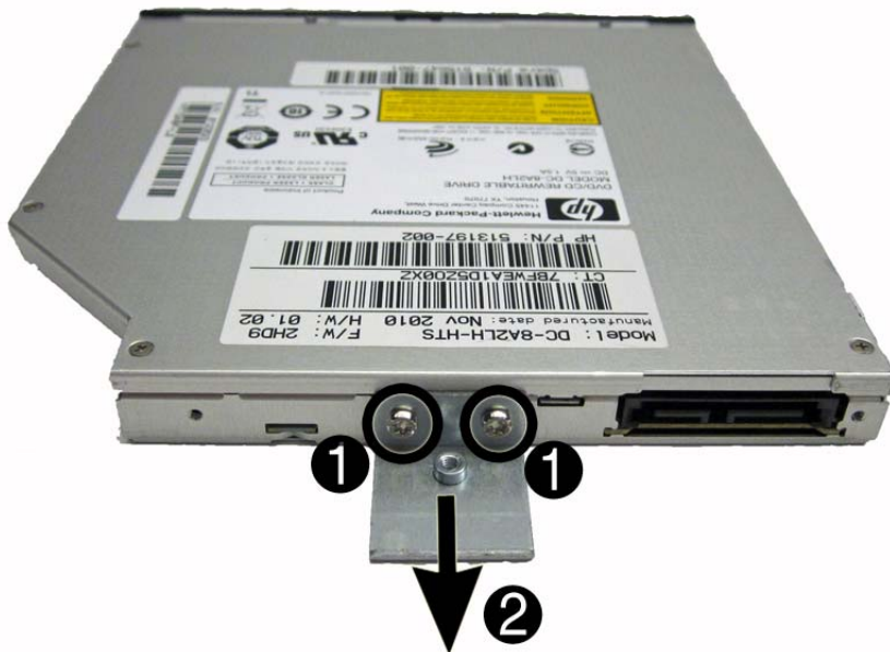
Figure 7-8 Removing the optical drive bracket
