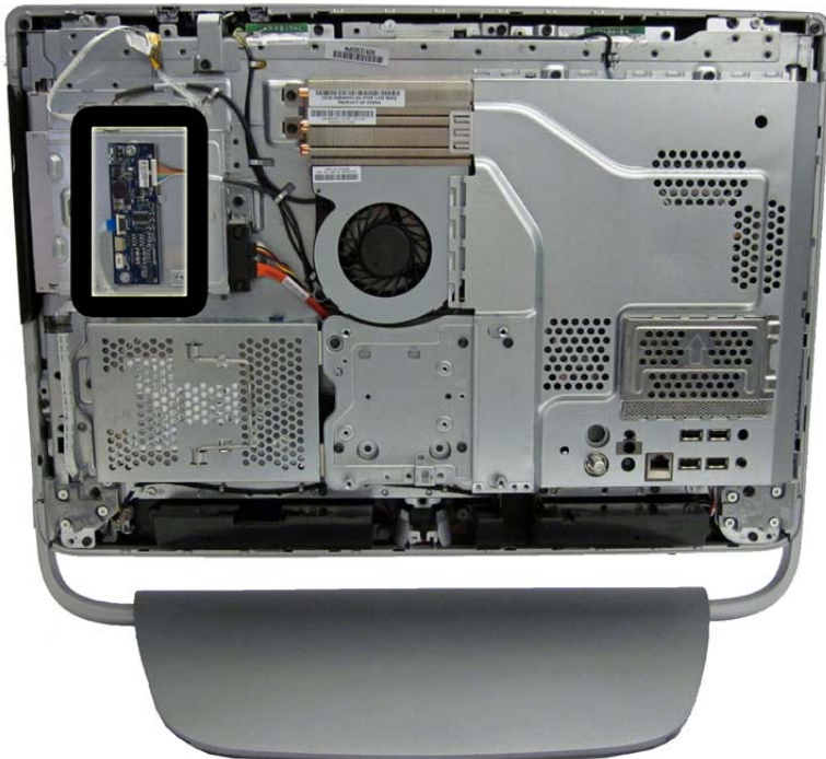
Figure 7-12 converter board location
