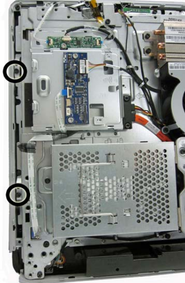
Figure 7-53 Removing the middle frame screws – left
