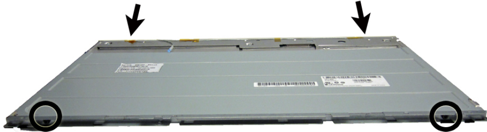
Figure 7-61 Display panel bracket location
