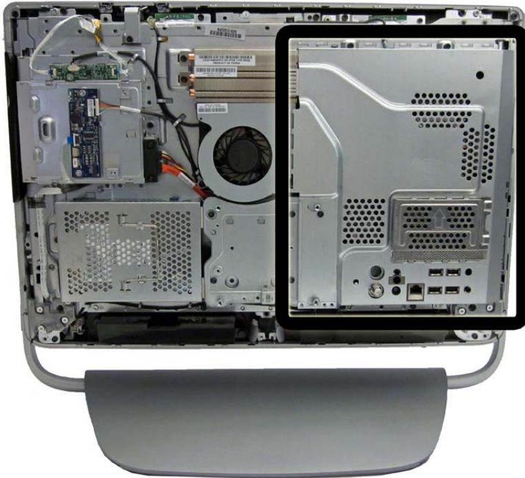
Figure 7-24 System board cover location
