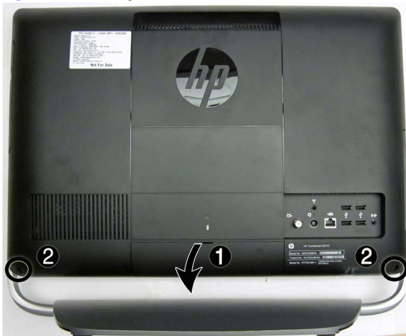
Figure 7-1 Removing the rear cover
