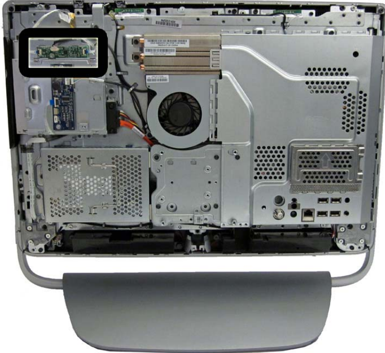
Figure 7-15 Touch controller board location
