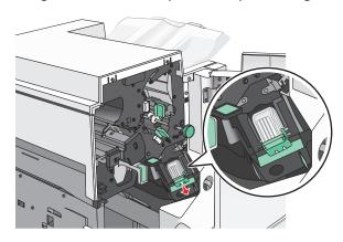
Use the metal tab to lift the staple guard, and then remove any jammed or loose staples.
