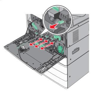
Slide the printhead wipers back into place.
