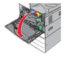
**2** Slide the release lever to the left to unlock the cover.
