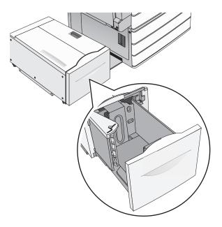
**2** Adjust the width guide as necessary.
