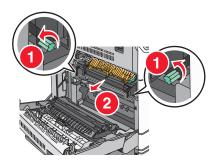
**3** Firmly grasp the jammed paper on each side, and then gently pull it down and out.
