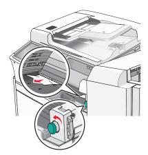
**Note:** If the paper jam on the right is difficult to remove, then rotate the knob counterclockwise.
