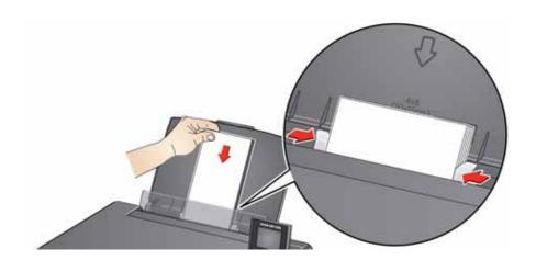
IMPORTANT: Always load the paper **short side first**. The printer automatically detects the orientation of the picture, whether it's portrait or landscape, and prints accordingly. If the photo paper is loaded in the wrong direction, the image will be cut off and the paper may jam. If the paper is loaded with the wrong side up, the image quality will be affected.
