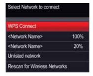
If there are more networks than can be shown on the LCD, a  $\nabla$  (page down) symbol appears in the bottom right of the display.
