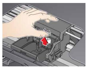
5. Lift the used printhead out of the carriage.
