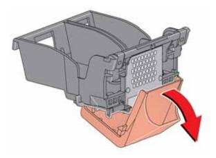
8. Place the new printhead into the carriage.
