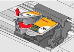
4. Unlatch the used printhead by lifting the button in the center of the carriage.
