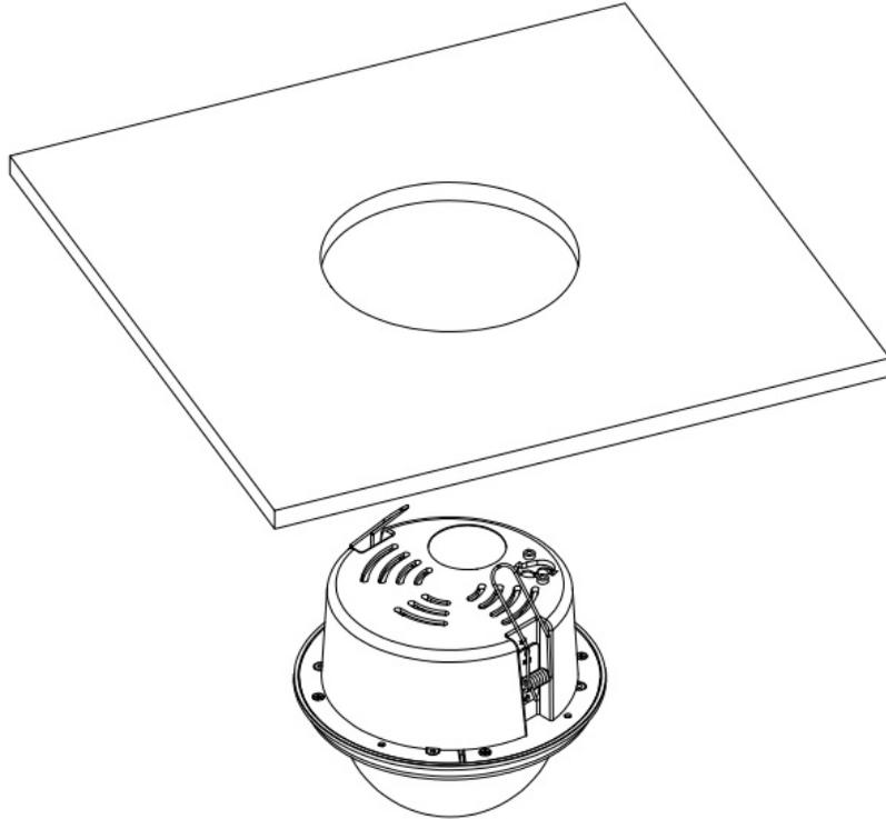
8. Preposition camera so it is facing approximately in the desired direction.
