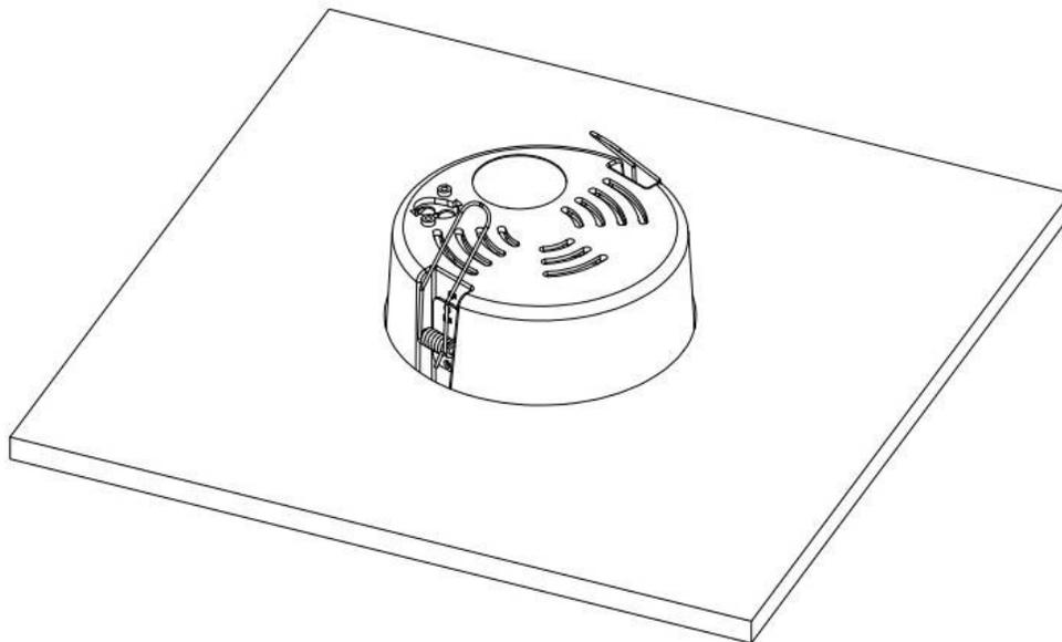
10. The spring tabs will open automatically to support the camera against the ceiling.
