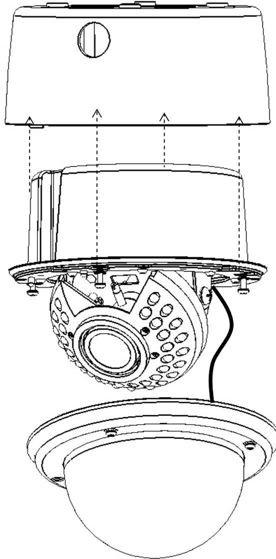
9. Attach video test cable to test point on rear of camera module. Aim and focus the camera. Remove test cable.
