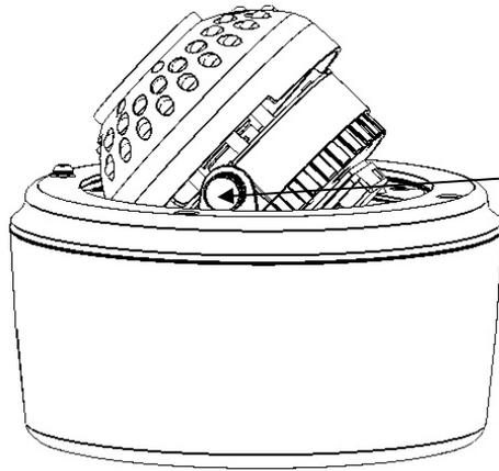
Loosen this screw manually to rotate the camera 180°
