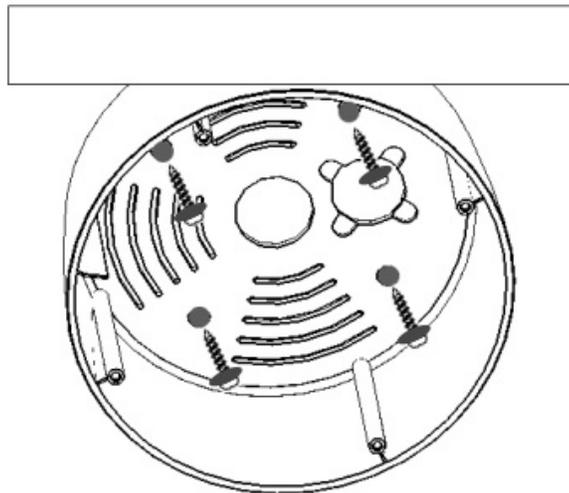
7. Attach power and video cables from source to cables from camera and push excess wire back into hole.
