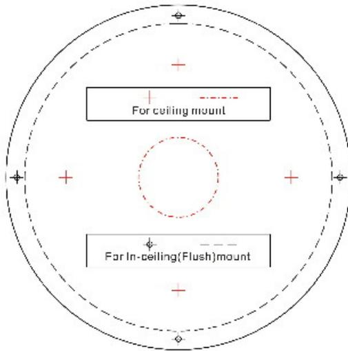
2. Use the appropriate tool to drill the INNER holes, and a clearance hole for the power and video wires.
