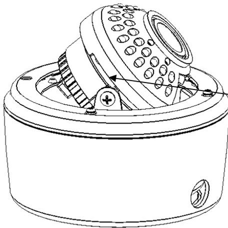
Use a screw driver to loosen this screw. Tilt the camera 180°
