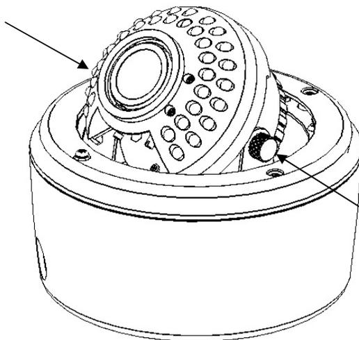
Hold the bracket at both sides of the camera. Rotate the entire camera 180°
