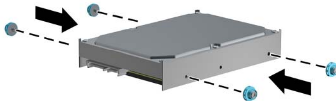
Figure 3-37 Installing Hard Drive Guide Screws
