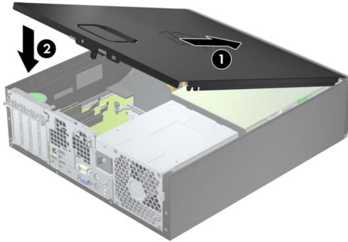
Figure 3-2 Replacing the Computer Access Panel
