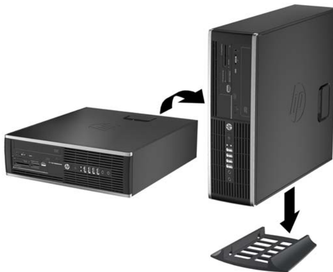
Figure 3-6 Changing from Desktop to Tower Orientation
