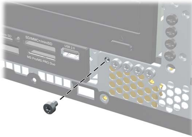
Figure C-11 Retrieving the Front Bezel Security Screw
