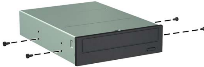
Figure 3-22 Installing Guide Screws in the Optical Drive
