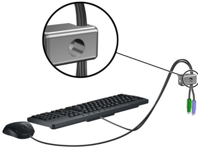
Figure C-7 Threading the Keyboard and Mouse Cables
