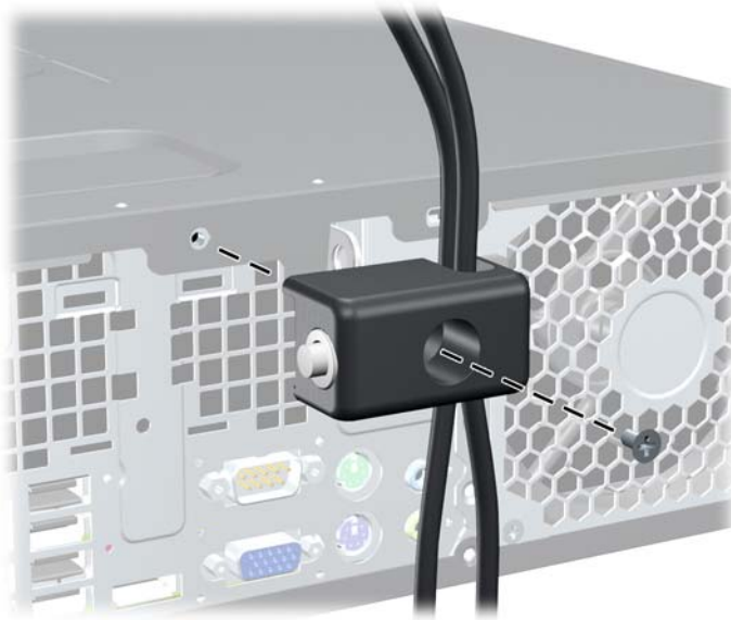
Figure C-8 Attaching the Lock to the Chassis
