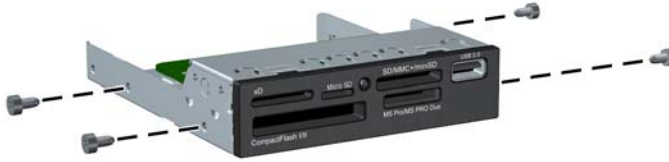
Figure 3-29 Installing Guide Screws (Media Card Reader Shown)
