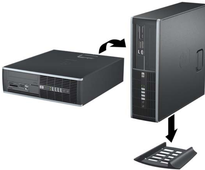
Figure 2-6 Changing from Desktop to Tower Orientation
