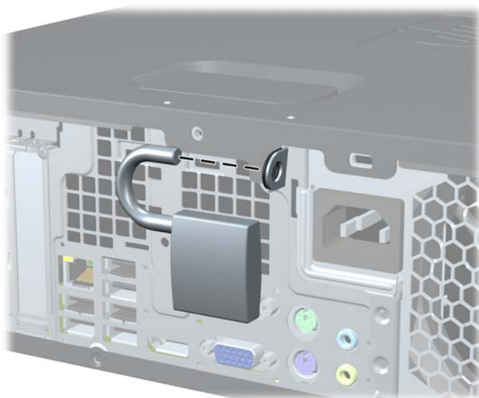
Figure C-2 Installing a Padlock
