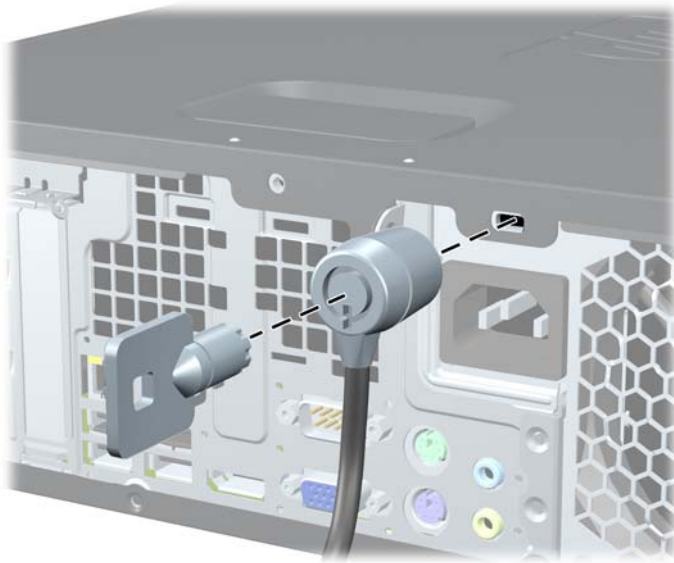
Figure C-1 Installing a Cable Lock
