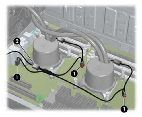
**b.** Disconnect the LCS cable harness inline connector (2), as shown in the previous figure.
