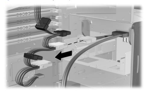
**8.** Disconnect the data cable from the hard drive (1), and from the system board connector (2), as shown in the following illustration.
