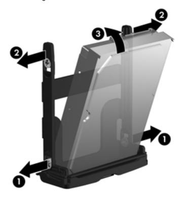
**6.** Carefully separate the upper hard drive carrier rails (2), and then rotate the drive upright (3), as shown above.
