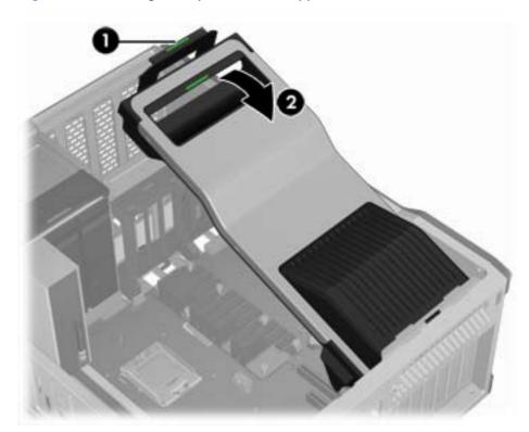
4. Disengage the expansion card support tabs from the rear chassis slots (1), and then lift the support from the chassis (2), as shown in the following figure.
