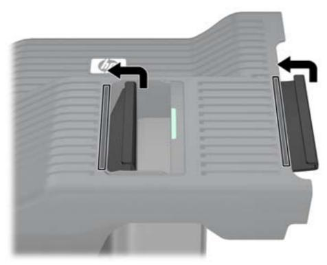
For proper installation, the LCS duct tabs sit above the surface of the main airflow guide as shown in the following figure.
