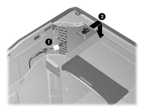
5. Slide the sensor back in its slot, push the sensor down, and then remove it from the chassis (2).
