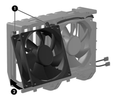
4. Guide the fan cable under the cable retention clamps as shown in the following figure.
