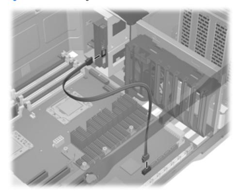
**9.** Disconnect the chassis power cable from the hard drive power connector as shown in the following figure.
