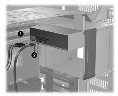
7. Connect the optical disk drive data cable to the next available SATA port on the system board as shown in the following figure.
