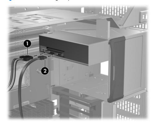
**6.** Lift the drive release latch at the green touch point (1), and gently slide the drive out of the chassis (2), as shown in the following figure.
