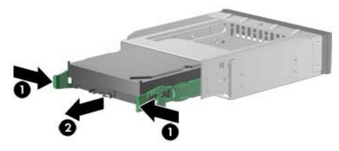
8. Carefully separate the rails (1), and remove the hard drive (2), as shown in the following figure.
