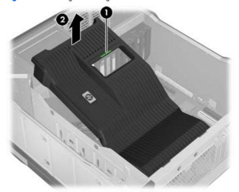
4. Disengage the airflow guide tabs from the rear chassis slots (1), and then lift the airflow guide from the chassis (2), as shown in the following figure.
