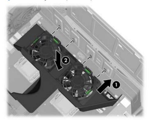
2. Press the release tabs at the green touch points with the index fingers, while grasping the side of the fan assembly with the remaining fingers. Carefully lower the fan assembly into the chassis until it clicks into place (2).
