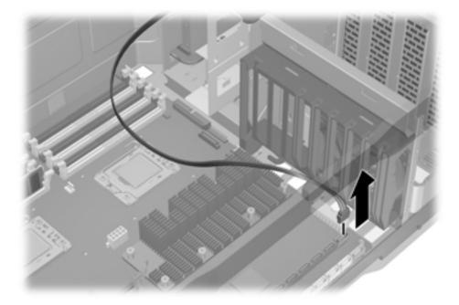
**6.** Disconnect the chassis power cable from the slot load optical drive power connector as shown in the following figure.
