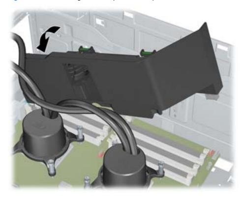
**b.** Install the memory fan assembly in the chassis (see <u>Installing the memory fans on page 157</u>).
