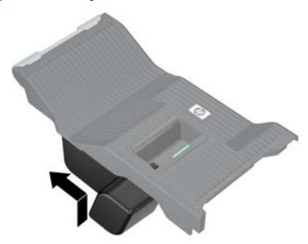
**b.** Slide the LCS air duct back into the airflow guide until it snaps into place as shown in the previous figure.
