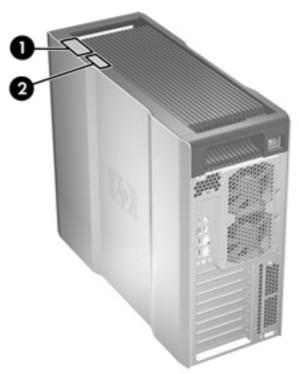
In general, the serial number labels can be found on the top panel or on the side of the workstation and at the rear of the workstation (your workstation may look different). Keep this number available when contacting customer service for assistance.
