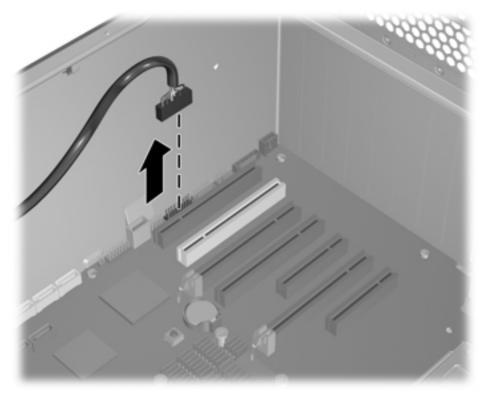
11. Guide the power switch cable assembly and cable out of the chassis.
