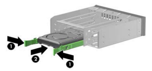
10. Lift and hold the drive release latch at the green touch point (1) while sliding the bracket into the optical bay (2), as shown in the following figure. When the front of the bracket is near its final position, release the latch, but continue to slide the bracket inward until the latch closes and engages the bracket.
