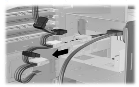
7. If a hard disk drive is installed, disconnect its power and data cables.
