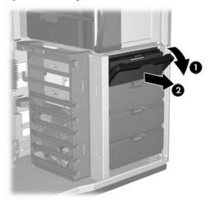
5. Set the hard drive in the carrier at an angle. Carefully separate the lower hard drive carrier rails (1), and then lower the drive between them, as shown in the following figure.
