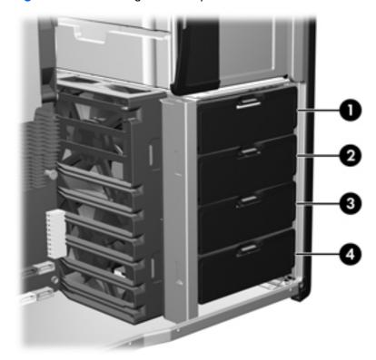
4. If there is a drive carrier in the drive slot, press the hard drive carrier release latch at the green touch point and rotate the handle outward (1). Pull the drive carrier out of the hard drive bay as shown in the following figure (2).
