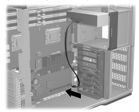
NOTE: If no SATA data port connector is available on the system board, check to see that all attached SATA cables are connected to active devices. An unused device can be disconnected to free up a SATA data port connector on the system board.
