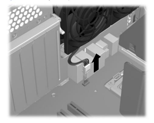
6. Use a Torx T-15 driver to remove the four rear system fan assembly Torx screws , and then remove the assembly from the rear of the chassis.
