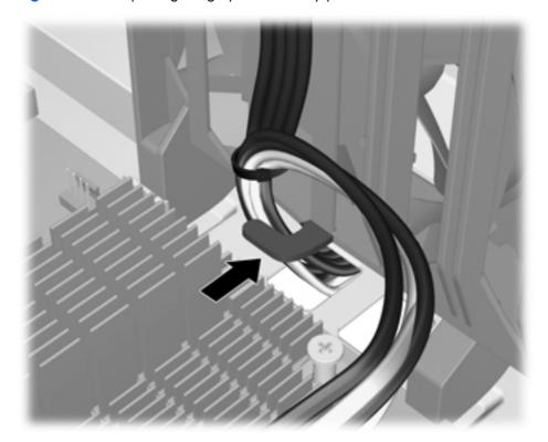
**7.** Clip the graphics auxiliary power connectors into the expansion card guide storage receptacles as shown in the following figure.
