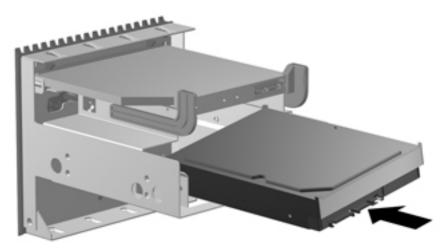
4. Rotate the hard drive flat, and adjust its position so the drive holes align with the carrier holes.
