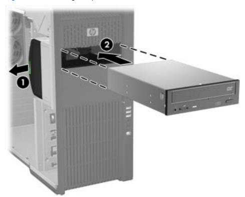
TIP: During installation the adjacent drive or filler may move slightly. You might have to slide and align both devices to get the release latch to close and engage both devices.
