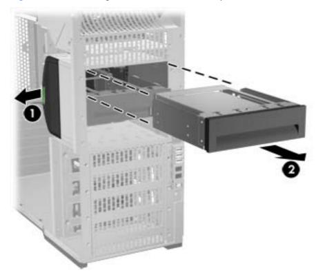
7. Carefully squeeze the ends of the rails together (1), and then slide the drive out of the carrier (2), as shown in the following figure.
