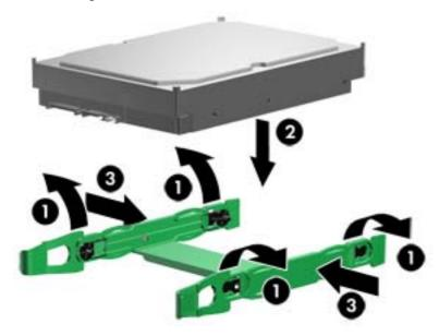
6. Slide the drive into the carrier until it snaps into place, as shown in the following figure.
