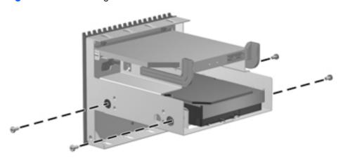
12. Remove the hard drive from the slot load optical drive carrier as shown in the following figure.
