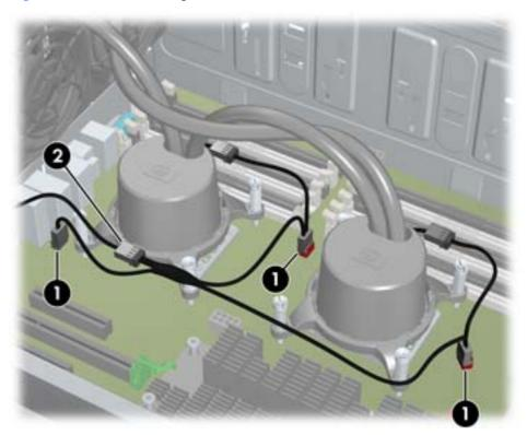
**b.** Connect the LCS cable harness inline connector to the rear system fan connector (2), as shown in the previous figure.
