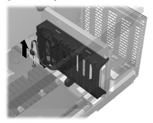
10. Press firmly on the two recessed green touch points on the top of the expansion card guide/front fan holder (1), as shown in the following figure.
