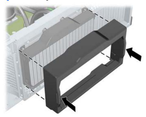
**b.** Press the cover onto the radiator until it snaps into place as shown in the previous figure.
