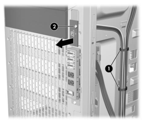
**9.** Remove the cable assembly by pulling cables through the lower right chassis wall opening and the front chassis wall opening.
