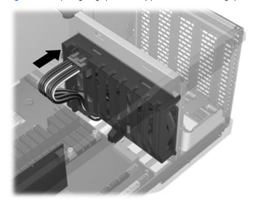
8. Connect the front system fan cable(s) to the system board as shown in the following figure. If there is only one fan, connect its cable to the inner-most connector.
