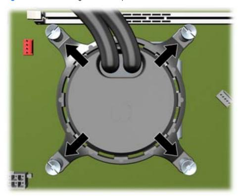
**b.** Gently twist the cold plate (1), and remove it from the retention ring (2), as shown in the following figure.
