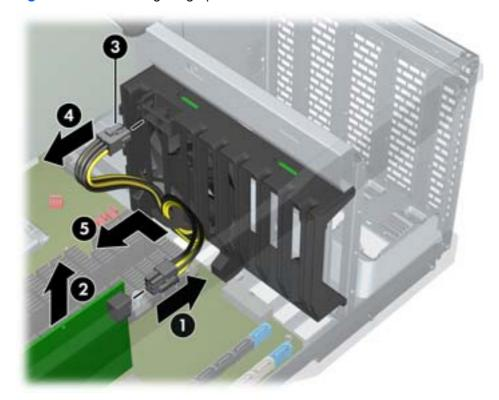
Disconnect the front system fan power cable from the system board as shown in the following figure.
