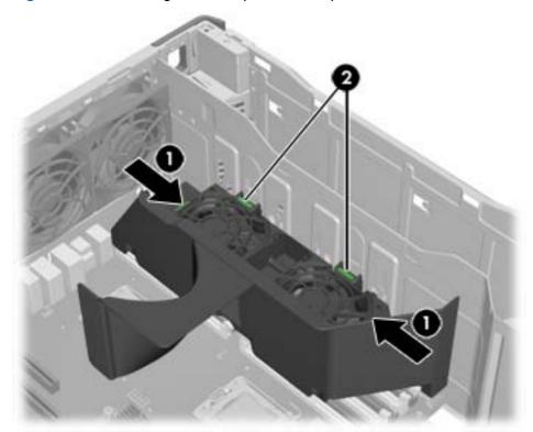
5. Lift the memory fan assembly upward, out of the chassis as shown in the following figure.
