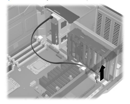
**7.** Disconnect the chassis power cable from the slot load drive power connector as shown in the following figure.
