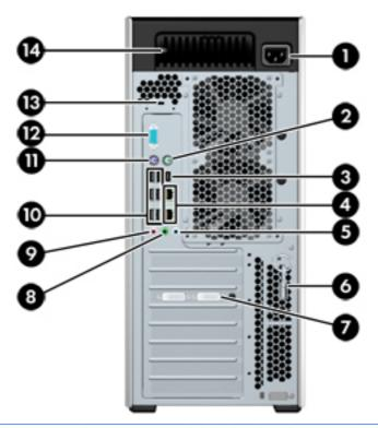
NOTE: The rear panel connectors are labeled with industry-standard icons and colors to assist in connecting peripheral devices.
