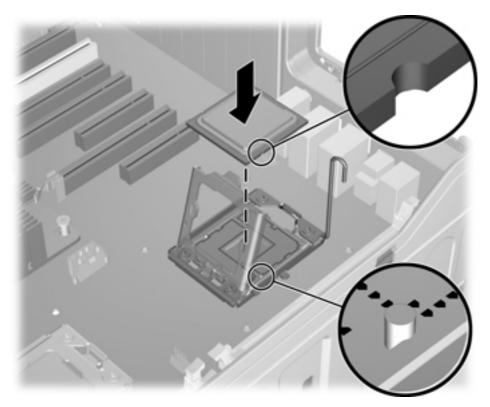
10. Close the CPU cover plate by lightly pressing down on the CPU cover plate while closing the socket lever.
