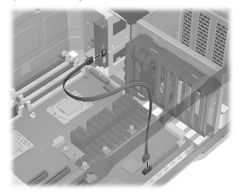
8. Connect the chassis power cable to the slot load optical drive power cable.
