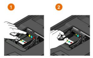
**Warning—Potential Damage:** Do not remove the old cartridges until you have the new cartridges available, or the ink remaining in the printhead may dry out and clog the nozzles.
