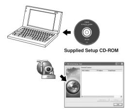
The VB Initial Setup Tool automatically detects the camera connected to the network, and displays its MAC address, IP address, and model name.
