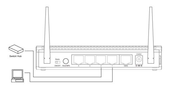
4. Connect the AC power adapter to the wall socket, then connect it to the Power socket of the router.
