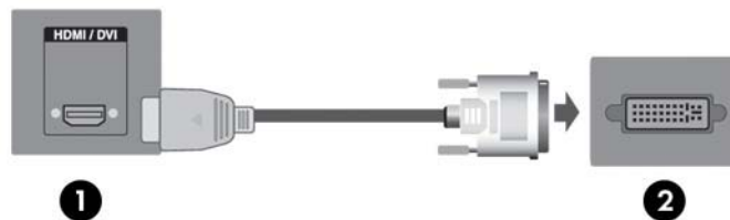
Figure 3-17 Connecting the HDMI to DVI Signal Cable
