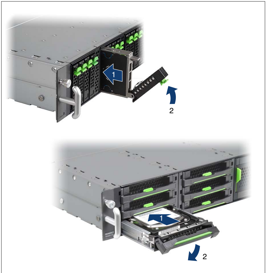
Figure 33: Installing the 2.5-inch and 3.5-inch HDD/SSD modules
