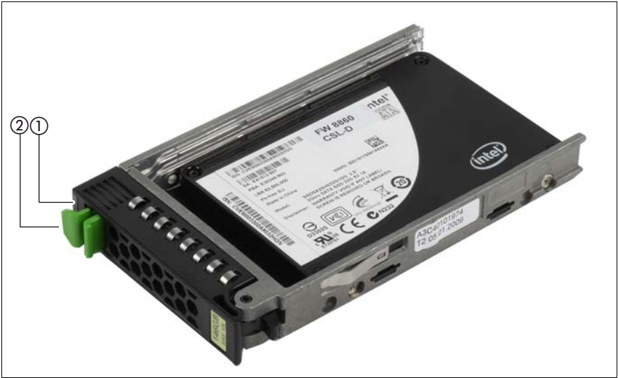
Figure 21: Indicators on the SSD modules
