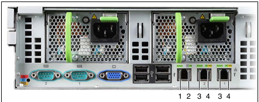
Figure 23: Indicators on the connection panel: LAN indicators
