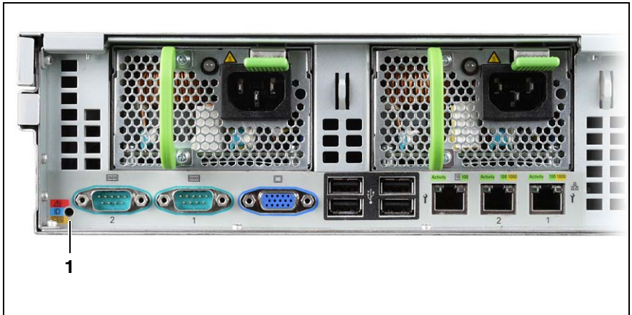
Figure 22: Indicators on the connection panel: Global Error/CSS/ID indicator
