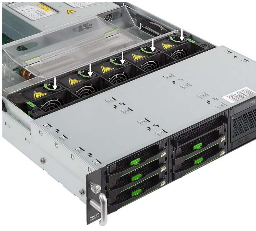
Figure 34: Arrangement of fans and the corresponding indicators
