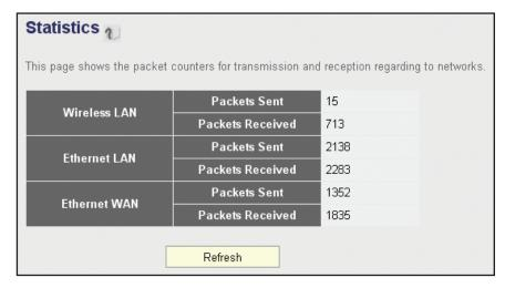
Refresh — Click to display the latest information. **NOTE**: The information is accumulative and is only reset after the router is restarted.
