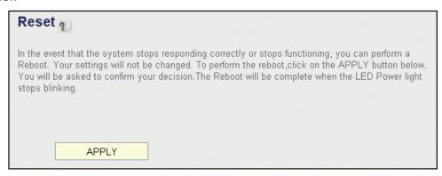
Apply — Click to reset the router. It will be operational again after a few minutes. **NOTE:** This function does not change any settings you have made. It simply restarts (reboots) the router — just as Start / Shut Down / Restart reboots your computer — freeing up memory and system resources for more stable operation.
