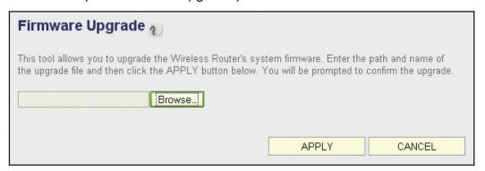
Browse — Click to locate the firmware file you've downloaded. If the file is in Zip (compressed archive) format, you need to uncompress it prior to the upgrade. Apply — Click to start the firmware upgrade process.
