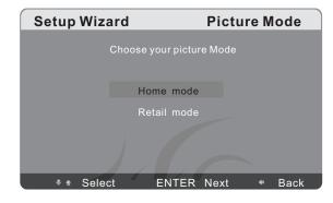
**4** Press ▲ or ▼ to select the **Home Mode** or **Retail Mode**, then press **ENTER**. Home Mode reduces the TV's total power consumption. The *Tuner Mode* screen opens.
