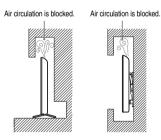
• Inadequate ventilation can lead to overheating of the TV and may cause damage to your TV or cause a fire.
