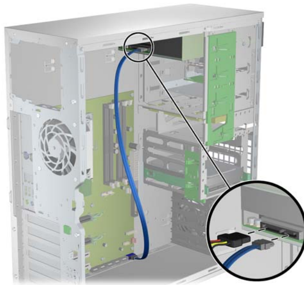
Figure 10-1 Connecting ODD power and data cables
