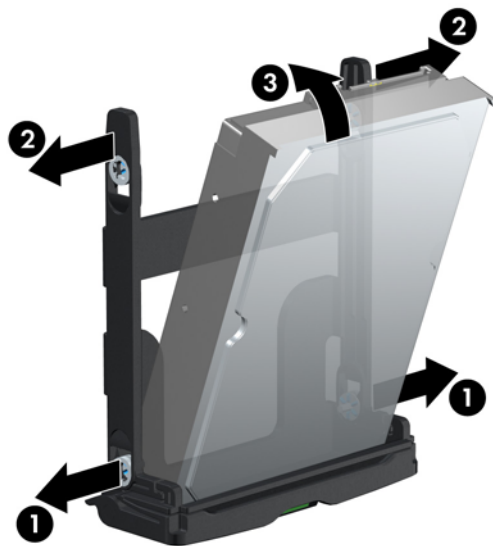
Figure 9-5 Installing the drive in the carrier
