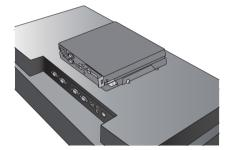
6 Use screws to secure the player and the Box Guide as shown below.
