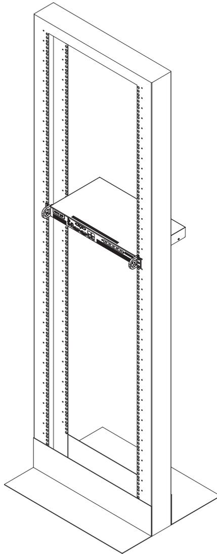
Figure 2-2. Installing the Chassis into a Telco Rack
