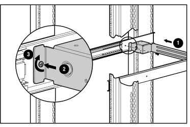
4. Attach the cable management arm to the right corner of the brace and secure it with two 6-32 screws.
