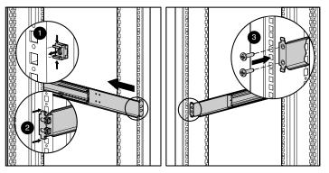
3. Attach the brace assembly to each mounting rail with the cable access hole facing the right side of the rack.
