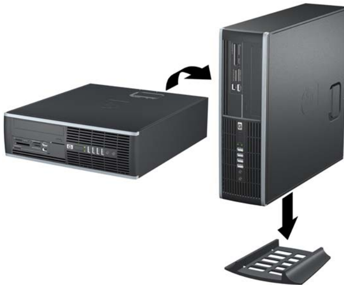
Figure 7 Changing from Desktop to Tower Orientation
