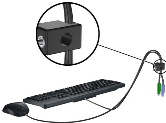
Figure 51 Threading the Keyboard and Mouse Cables
