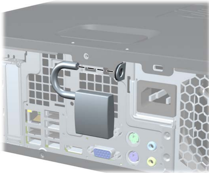
Figure 49 Installing a Padlock
