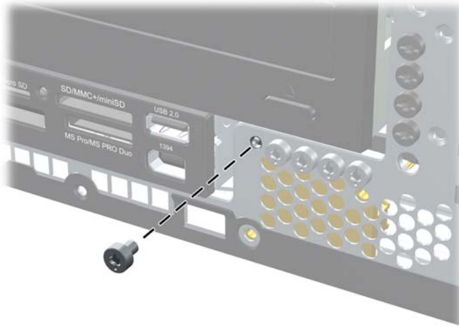
Figure 54 Retrieving the Front Bezel Security Screw
