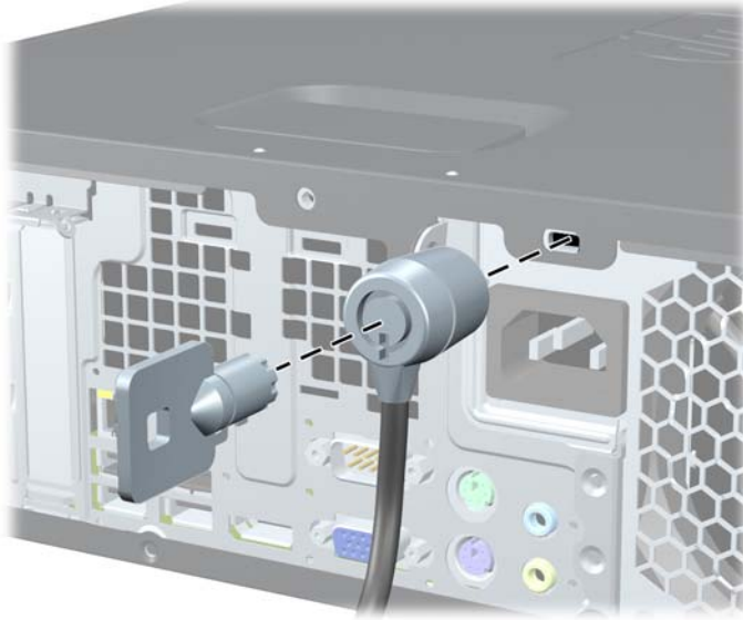
Figure 48 Installing a Cable Lock
