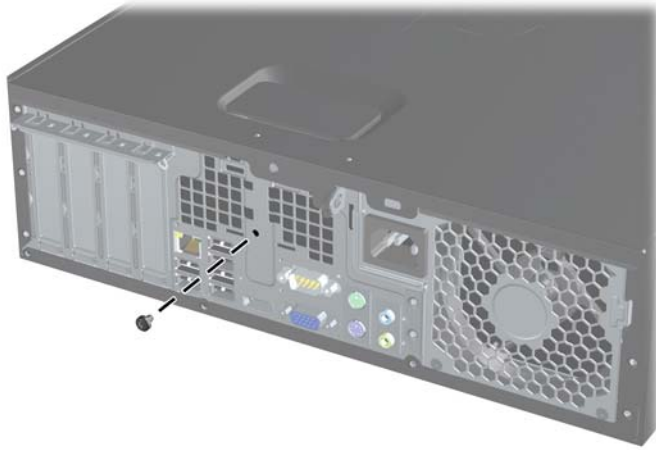
Figure 1 Removing the Smart Cover Lock Screw
