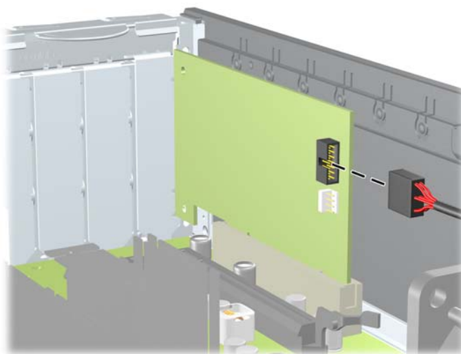
Figure 28 Disconnecting the Media Card Reader 1394 Cable
