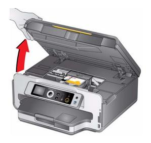
The ink cartridges are located in the printhead.
