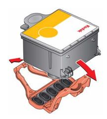
6. Insert the ink cartridge into the printhead.
