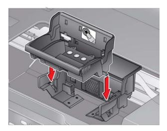
9. Push firmly against the target label of the printhead until you hear a loud snap.
