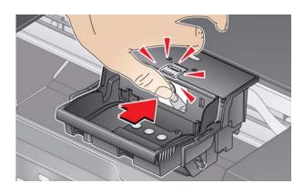
10. Insert the black ink cartridge into the printhead.
