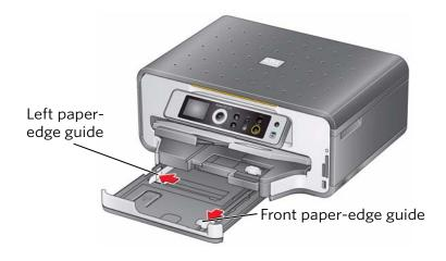
4. Press the paper tray extender, and pull the paper tray forward until it is fully extended.
