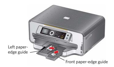
4. Fan and stack the photo paper, then insert it (short side first) into the tray with the **logo side facing up** and the glossy side down.
