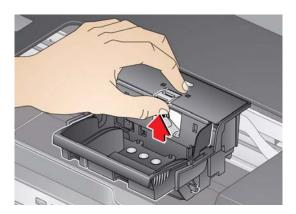
5. Lift the used printhead out of the carriage.
