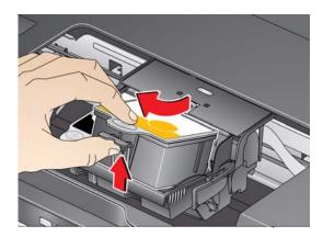
4. Unlatch the used printhead by lifting the button in the center of the carriage.
