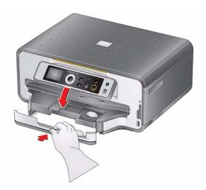
9. Pull out the output tray extender until it is fully extended, but do not lift the paper stop.
