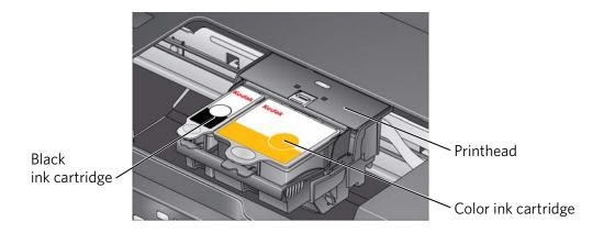
3. Pinch the tab on the ink cartridge and lift it out of the printhead.
