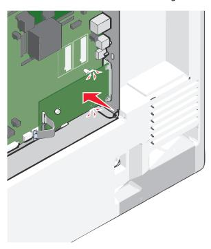
Insert the long thumbscrew and turn it clockwise, enough to hold the ISP in place, but do not yet tighten the thumbscrew.
