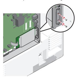
**c** Insert the plug of the printer hard disk interface cable into the receptacle of the system board.
