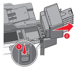
**2** Open the finisher door, and then removed the jammed paper.
