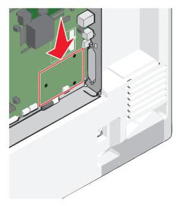
**Note:** If an optional ISP is currently installed, then the printer hard disk must be installed onto the ISP. To install a printer hard disk onto the ISP:
