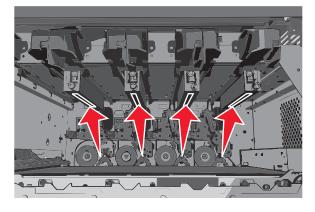
4 Clean the lenses using compressed air.
