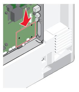
**4** Remove the printer hard disk.
