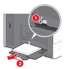
**Warning—Potential Damage:** Pulling the paper out, without pushing the paper pick tab first, may cause the paper pick tab to break.
