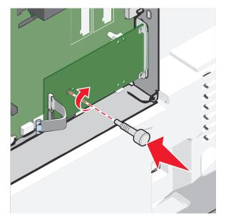
Attach the two provided screws to secure the ISP mounting bracket to the system board cage.
