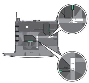
2 Squeeze and then slide the width guide to the correct position for the paper size you are loading.
