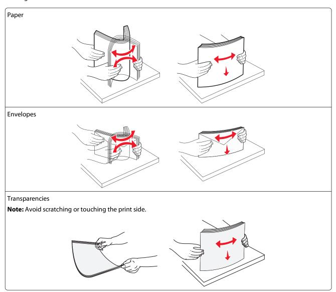
**4** Push the paper pick tab, and then load the paper or specialty media. Slide the stack gently into the multipurpose feeder until it comes to a stop, and then release the paper pick tab.
