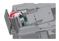
Remove the pick roller assembly.
