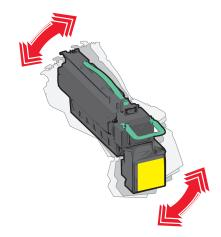
**6** Remove the red packing strip from the new cartridge.
