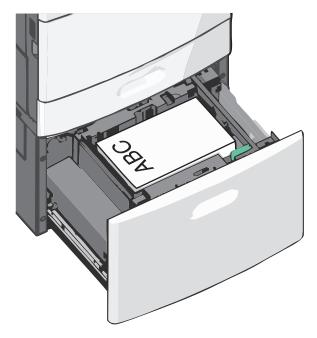
**Note:** Make sure the paper is below the maximum fill line located on the edge of the paper tray. Overloading the tray can cause paper jams.
