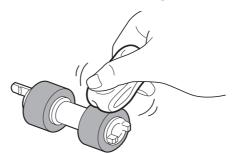
**4.** Turn the short tab (1) of the feed roller to the right and slowly push it onto the shaft of the paper tray.
