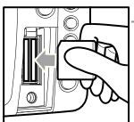
Inserting an SD into the Card Slot
