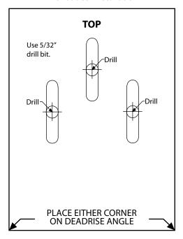
**NOTE:** If you are reproducing or printing this template from an electronic file, start with the following print settings: Scale = None, Paper = 8.5 x 11 inches, Layout = Portrait. Confirm that the template matches the transducer bracket slots and adjust the print as needed.
