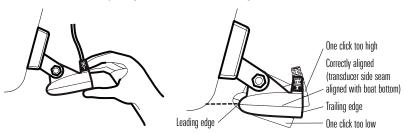
7. Adjust the transducer assembly vertically, until the seam on the leading edge of the transducer (the edge closest to the transom of the boat) is level and just slightly below the hull.
