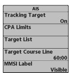
**AIS Submenu:** The AIS submenu allows you to track targets, receive alerts when targets are within the distance you set, and display targets in Chart Views. In Bird's Eye View, only the position will be displayed.
