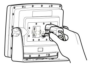
**NOTE:** You may wish to dress the cabling with nylon wire ties in order to hold the cables together and create a cleaner assembly.
