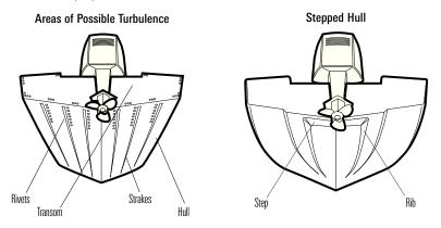
The best way to locate turbulence-free water is to view the transom while the boat is
