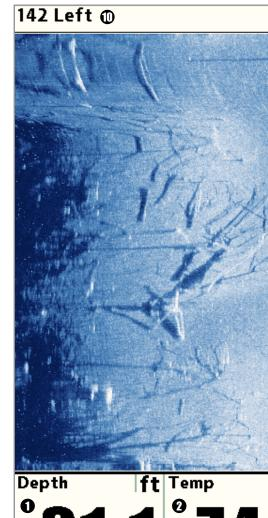
Side Imaging® Range – Images shown on the right side of the screen are located on the right side of your boat, and images shown on the left side of the screen are located on the left side of your boat. In this illustration, the sonar is pinging 142 feet on each side.
