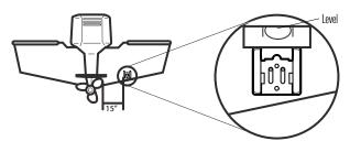
Find a turbulence-free location at least 15" from the propeller(s) and not in line with trailer bunks or rollers.
