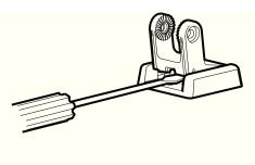
**NOTE:** If the pivot assembly is snapped closed over the mounting bracket, use a flat head screwdriver or similar tool to gently pry the assembly away from the mounting bracket.
