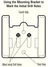
Continue to hold the bracket on the transom of the boat, and use a pencil or marker to mark where to drill the two mounting holes. Mark the drill holes near the top of each slot, making sure that your mark is centered in the slot.
