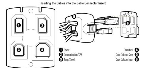
11. Line up the cable collector insert and cover, with the keying feature, then slide the cover into place on the insert.
