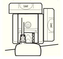
**NOTE:** The transducer has a natural downward slant of 4-5 degrees from leading edge (closest to the boat transom) to trailing edge (farthest away from the boat). Looking at the back of the transducer, the seam should be slightly below the bottom of the hull.
