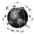
GPS uses a constellation of satellites that continually send radio signals to the earth. The GPS receiver on your boat receives signals from satellites that are visible to it. Based on time differences between each received signal, the GPS receiver determines its distance to each satellite. With distances known, the GPS receiver mathematically triangulates its own position. With once per second updates, the GPS receiver then calculates its velocity and bearing.
