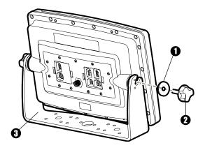
**Supplies:** In addition to the hardware supplied with your control head, you will need a powered hand drill and various drill bits, various hand tools, including a Phillips head screwdriver, a socket wrench and a flat head screwdriver, a marker or pencil, safety glasses and dust mask, and marine-grade silicone sealant.
