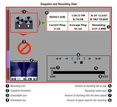
**NOTE:** For snapshots and recordings, the indicator bar has several states: during recording, the amount of space remaining on the SD card is indicated on the status bar. During playback, the amount of time/memory remaining to play is indicated on the status bar. When a snapshot thumbnail is highlighted, the amount of room remaining on the SD card is indicated.
