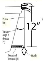
**NOTE:** It is important to take your measurement in the figure showing **Measuring the Transom Angle**, from exactly 12 inches down from the top of the transom.
