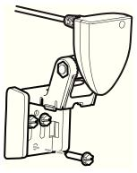
Fully Tighten All Three Mounting Screws
