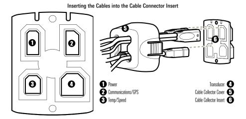
8. Line up the cable collector insert and cover, with the keying feature, then slide the cover into place on the insert.
