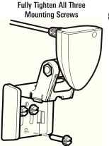
8. Re-position the transducer assembly against the transom of the boat, then hand-install all three screws. Make sure that the transducer location and the pivot angle have not changed, then fully tighten all three mounting screws. Snap the pivot back down. If you have performed the preceding procedures correctly, the transducer should be level and at the right height for optimal operation.
