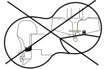
**Obstructed View:** The transducer is too close to motor turbulence, and the Side Imaging® view is blocked by the motor. The view cannot extend from side-to-side.
