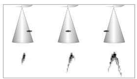
Transducer Cone and Fish Arches
