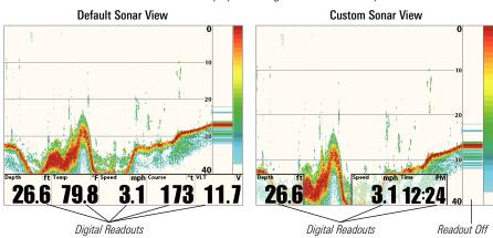
**NOTE:** When the readout under the water column is turned off (as shown in the illustration), the sonar display will expand to fill the screen.
