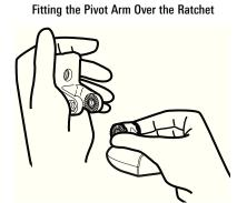
3. Put the pivot bolt through the assembly to hold it in position and loosely install the nut, but do NOT tighten the nut at this time. Insert the pivot arm assembly into the mounting bracket. Do NOT snap the assembly closed, as you will need to access the mounting bracket in the next step.
