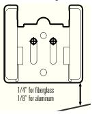
**NOTE:** If you have a flat-bottomed aluminum boat, some additional adjustment may be needed to accommodate the rivets on the bottom of the boat (i.e. the gap may need to be a little smaller than 1/8"). This will help you to avoid excessive turbulence at high speeds.
