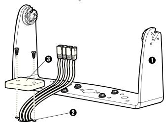
9. Thread the cables through the opening in the back of the cable collector cover.
