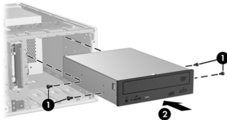
Figure 5-22 Installing the optical drive
