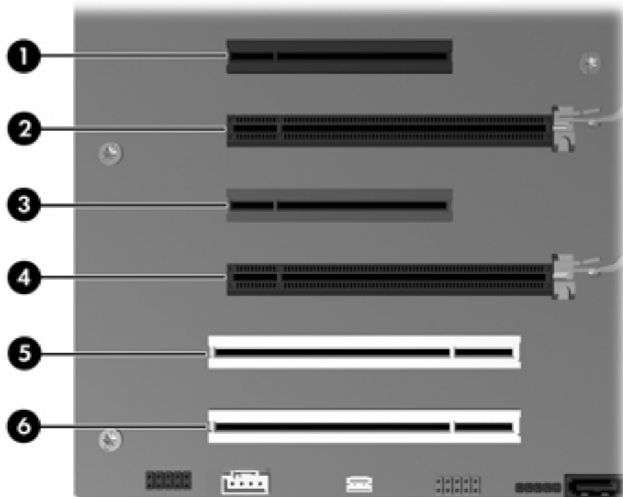
Figure 5-48 Identifying expansion card slots
