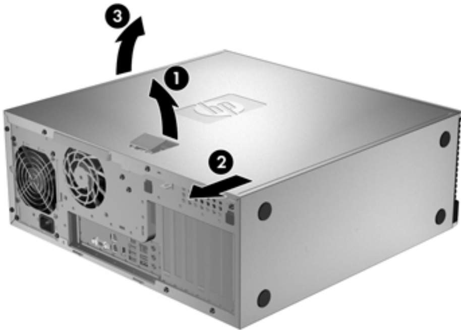
Figure 5-4 Removing the side access panel
