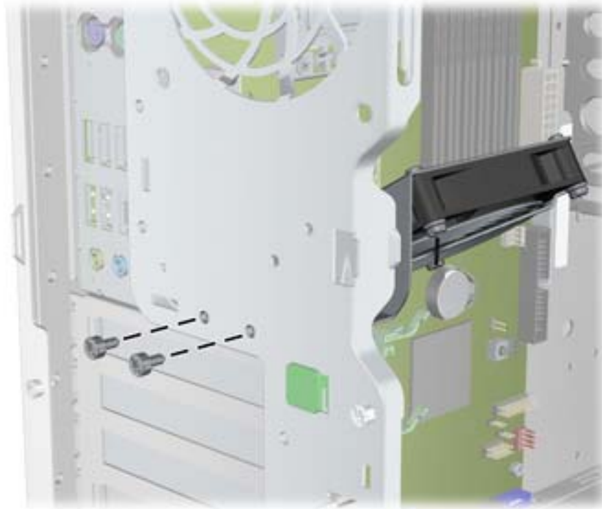
Figure 5-77 Fastening the LCS VR fan
