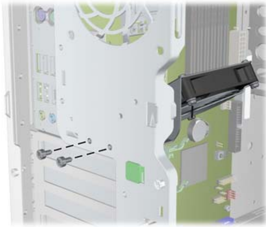
Figure 5-60 Removing the LCS VR fan assembly
