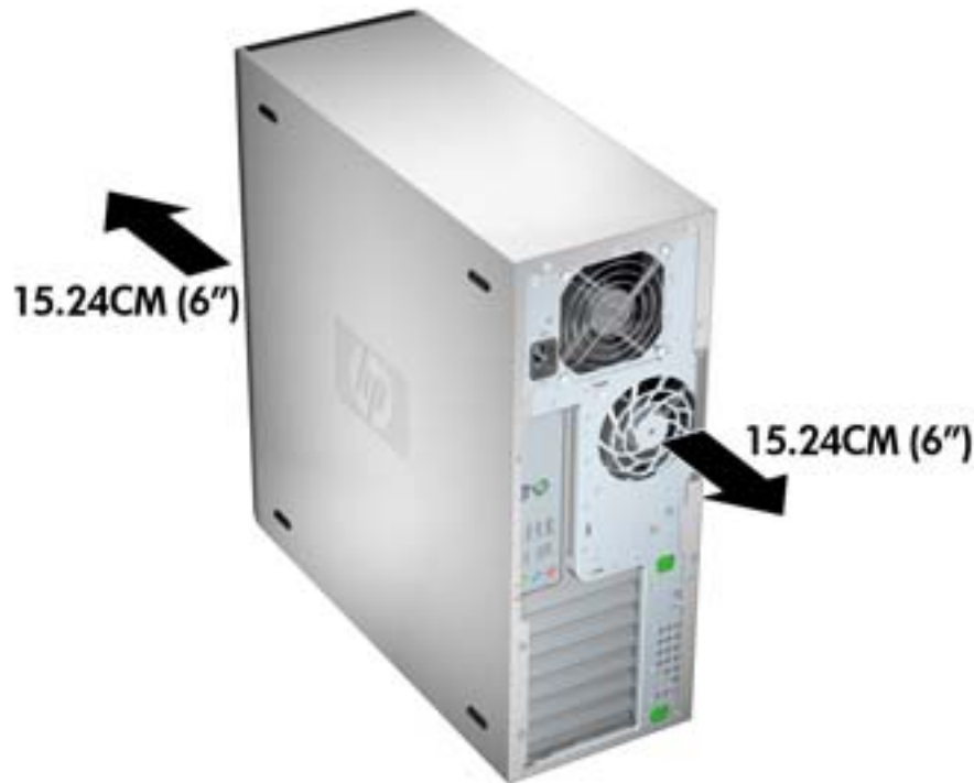
Figure 1-6 Proper workstation ventilation
