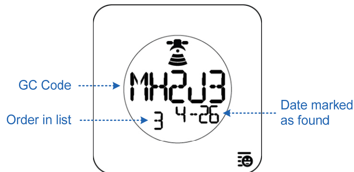
Figure 18: An example of a found geocache listing on the found list page
