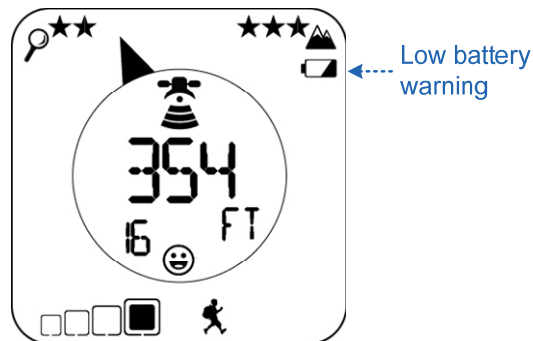
Figure 19: The low battery warning symbol. You should change batteries ASAP if you see it!
