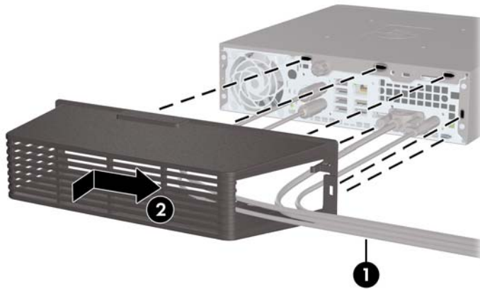
Figure 6-28 Installing a Port Cover
