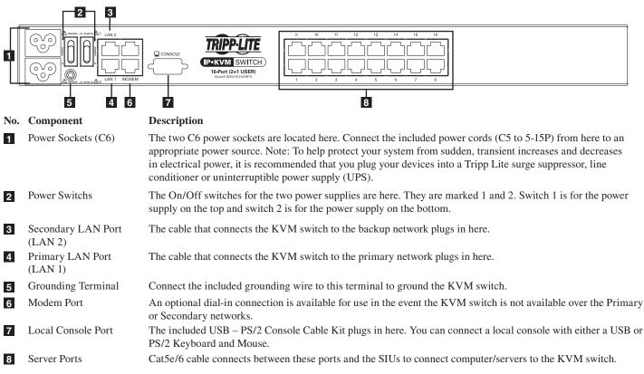
Note: The figure above shows the rear panel of a B064-032-04-IPG or B064-032-02-IPG. The B064-016-04-IPG and B064-016-02-IPG differ in that it only has a single block of 16 KVM ports.
