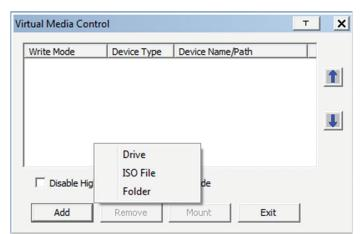
*Note: If your media source is USB 1.1, check the* Disable High Speed USB Operation Mode *checkbox*.
