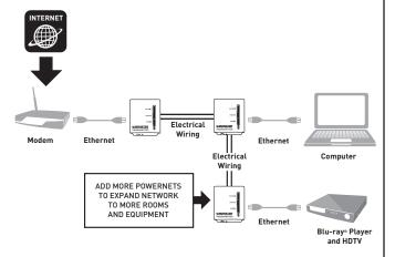
NOTE: The PLN 100 needs to pair with at least one other PLC device, such as the PowerNet 200, to create a working system.
