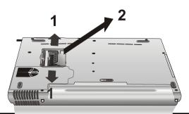
4. Pull upwards on the card and then slide the card out (2).
