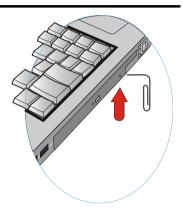
The CD disk tray should eject immediately. This procedure can also be used to remove a CD from the drive when the notebook is powered off.
