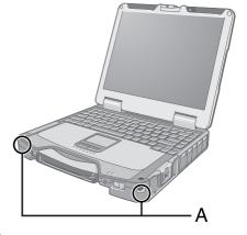
Use the tether to attach the stylus to the computer so you will not lose it. There are holes (A) to attach it.
