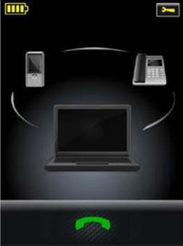
Figure 36: A disconnected target phone is shown greyed out on the touchscreen
