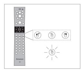
The air mouse buttons are: Left air mouse button, Air mouse On/Off button, Right air mouse button.
