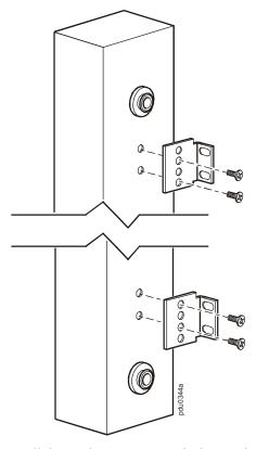
2. Install the Rack PDU on a vertical mounting rail in your rack or enclosure using the supplied screws and caged nuts with your enclosure.
