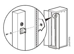
**Horizontal mounting.** You can mount the Rack PDU in a 19-inch NetShelter or other EIA-310-D standard 19-inch rack:
